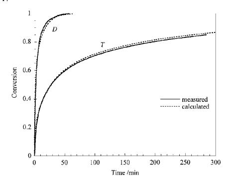
Fig. 4. Measured and calculated conversion versus time for two different uranium dioxides, D and T.
