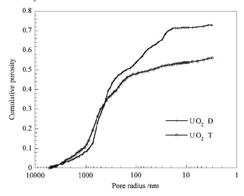
Fig. 5. Mercury intrusion curves for two uranium dioxide samples.
