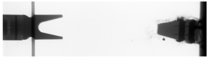
Fig. 8. X-ray picture of the armatures as they leave the barrel.
