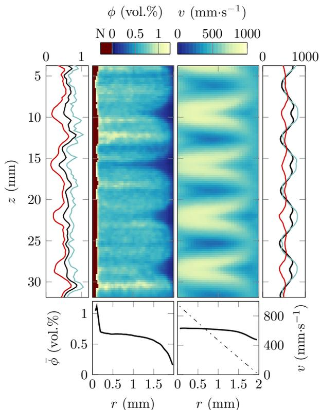
FIG. 9. Same as Fig. 8 for the turbulent Taylor vortex flow of a dilute suspension of PS-2 spheres in water sheared at  $\dot{\gamma} = 500 \text{ s}^{-1}$ . The global particle volume fraction is  $\phi_0 = 0.5\%$ . The ultrasonic data were time-averaged over 5,000 successive acquisitions performed within 0.25 s.
