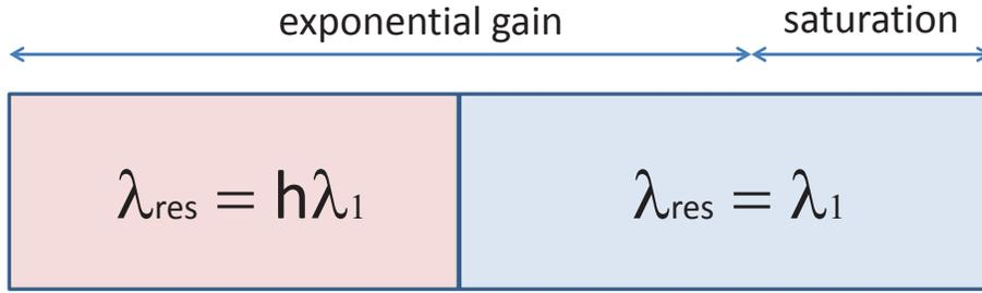
FIG. 3: Conceptual scheme of a harmonic lasing self-seeded FEL
