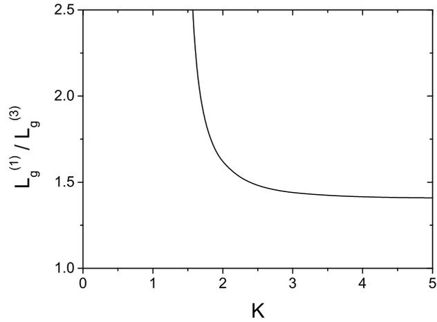
FIG. 2: Ratio of the gain length of the retuned fundamental to the gain length of the third harmonic (3) for lasing at the same wavelength versus rms undulator parameter  $K$ . The ratio is derived in the frame of the three-dimensional theory for an optimized beta-function and negligible energy spread [9].
