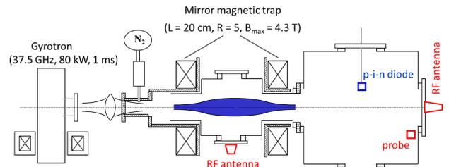
FIG. 1. The schematic view of the SMIS-37 setup.
