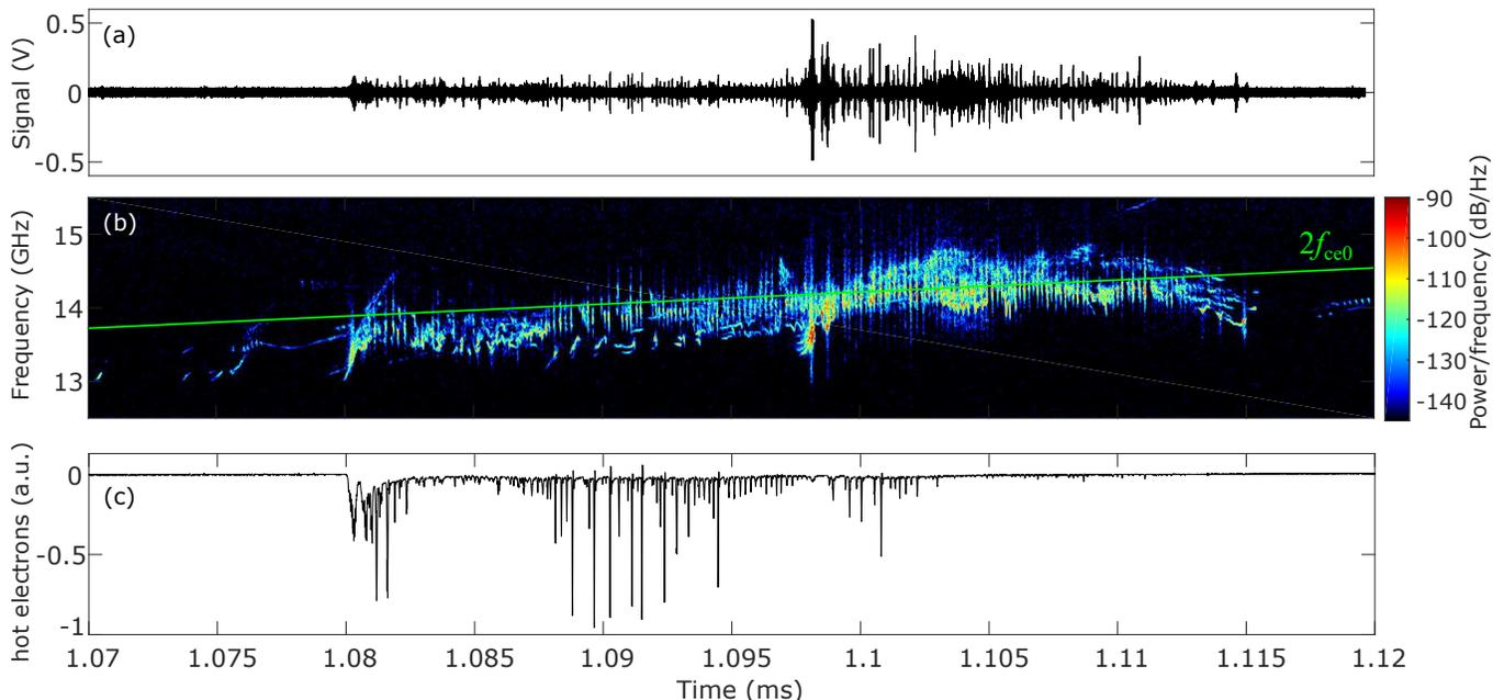
FIG. 6. (a,b) Series of quasiperiodic bursts of plasma emission under double plasma resonance condition and (c) synchronous precipitations of energetic electrons from the trap. The value of  $2f_{ce0}$  at the trap center is shown by a green solid curve on the dynamic spectra.
