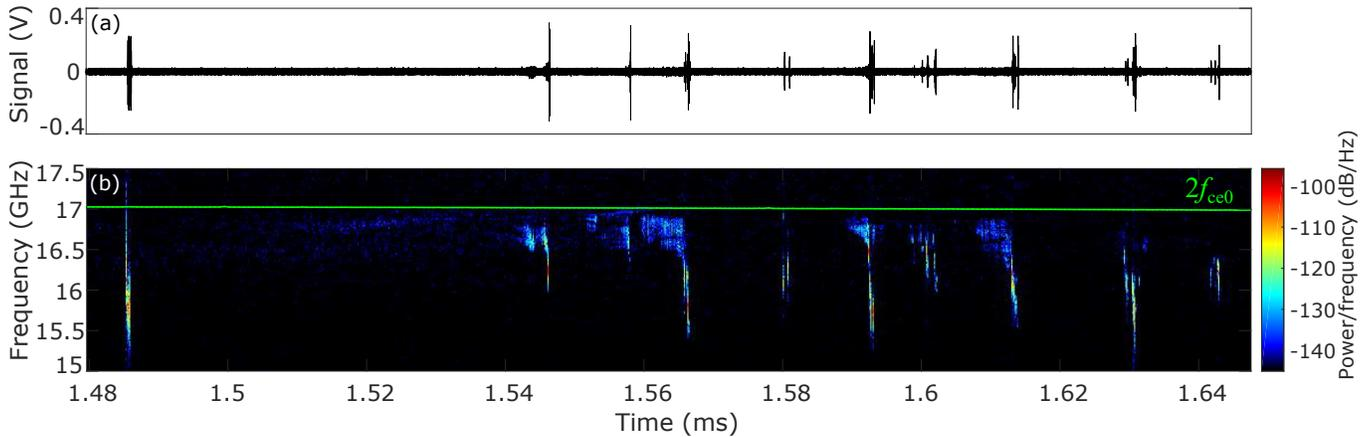
FIG. 7. Series of quasiperiodic bursts of plasma emission in decaying plasma. The value of  $2f_{ce0}$  at the trap center is shown by a green solid curve on the dynamic spectra.
