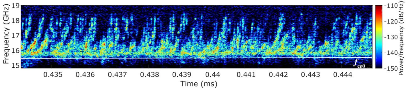
FIG. 4. Zoom of spectrum shown in Fig. 3(b). Here the periodic fast rising tones are clearly visible.
