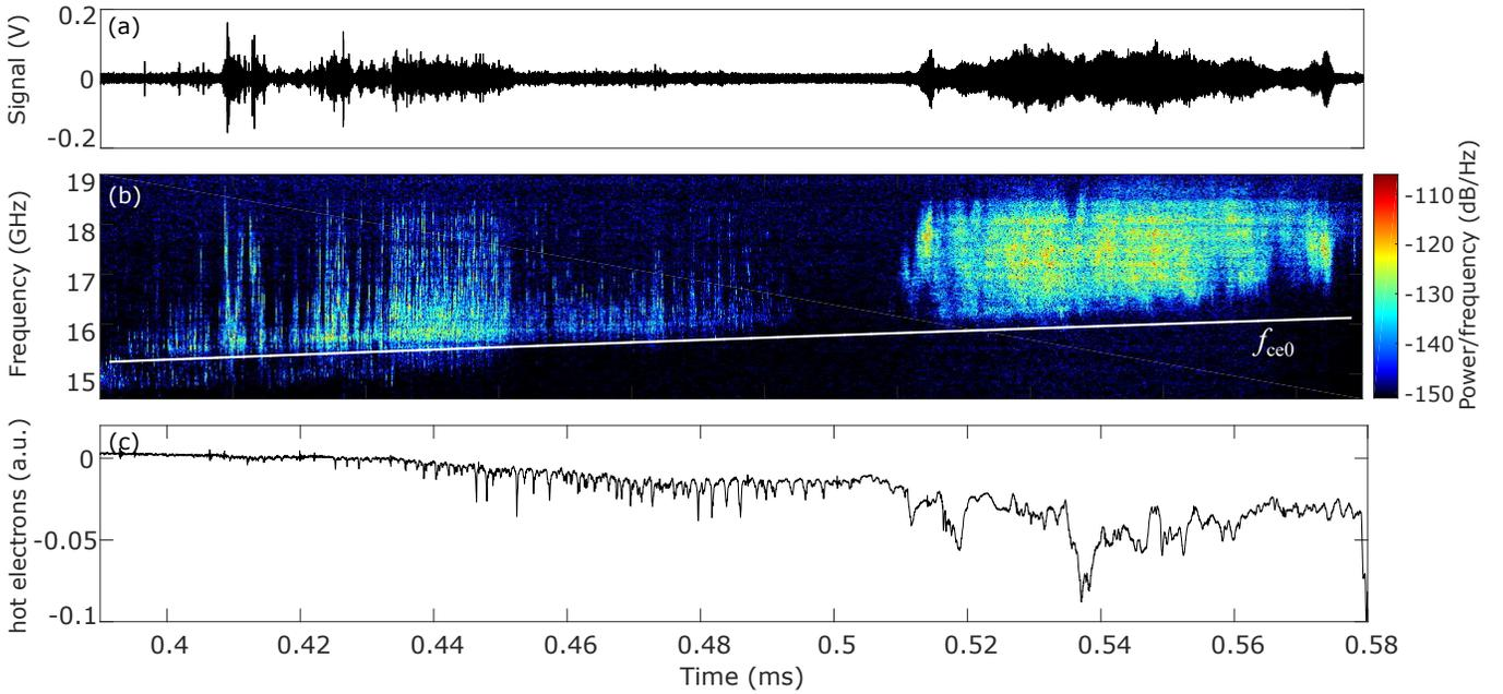
FIG. 3. (a) Waveform and (b) its dynamic spectrum of plasma microwave emission at the start-up stage, (c) the corresponding signal from the hot electron detector. The value of the electron gyrofrequency  $f_{ce0}$  at the trap center is shown by a white solid curve on the dynamic spectra.
