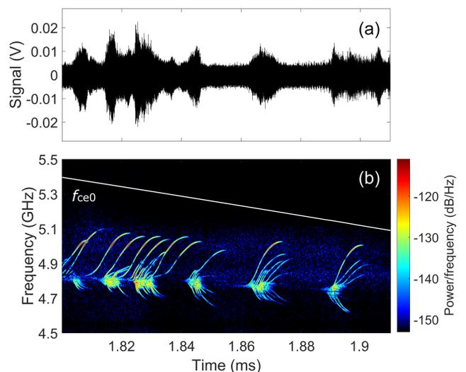
FIG. 8. Electric field oscillations (a) and corresponding dynamic spectrum (b) for the microwave emission during the late decay stage.
