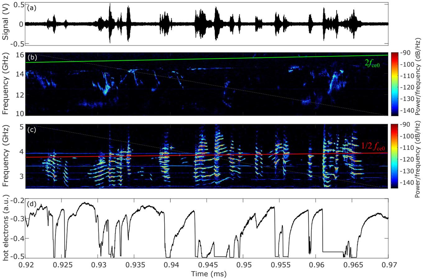
FIG. 5. (a) Waveform and (b,c) its dynamic spectrum of plasma microwave emission during the stationary ECR discharge, (d) the signal from the hot electron detector. The values of  $f_{ce0}/2$  and  $2f_{ce0}$  at the trap center are shown by solid curves on the dynamic spectra.
