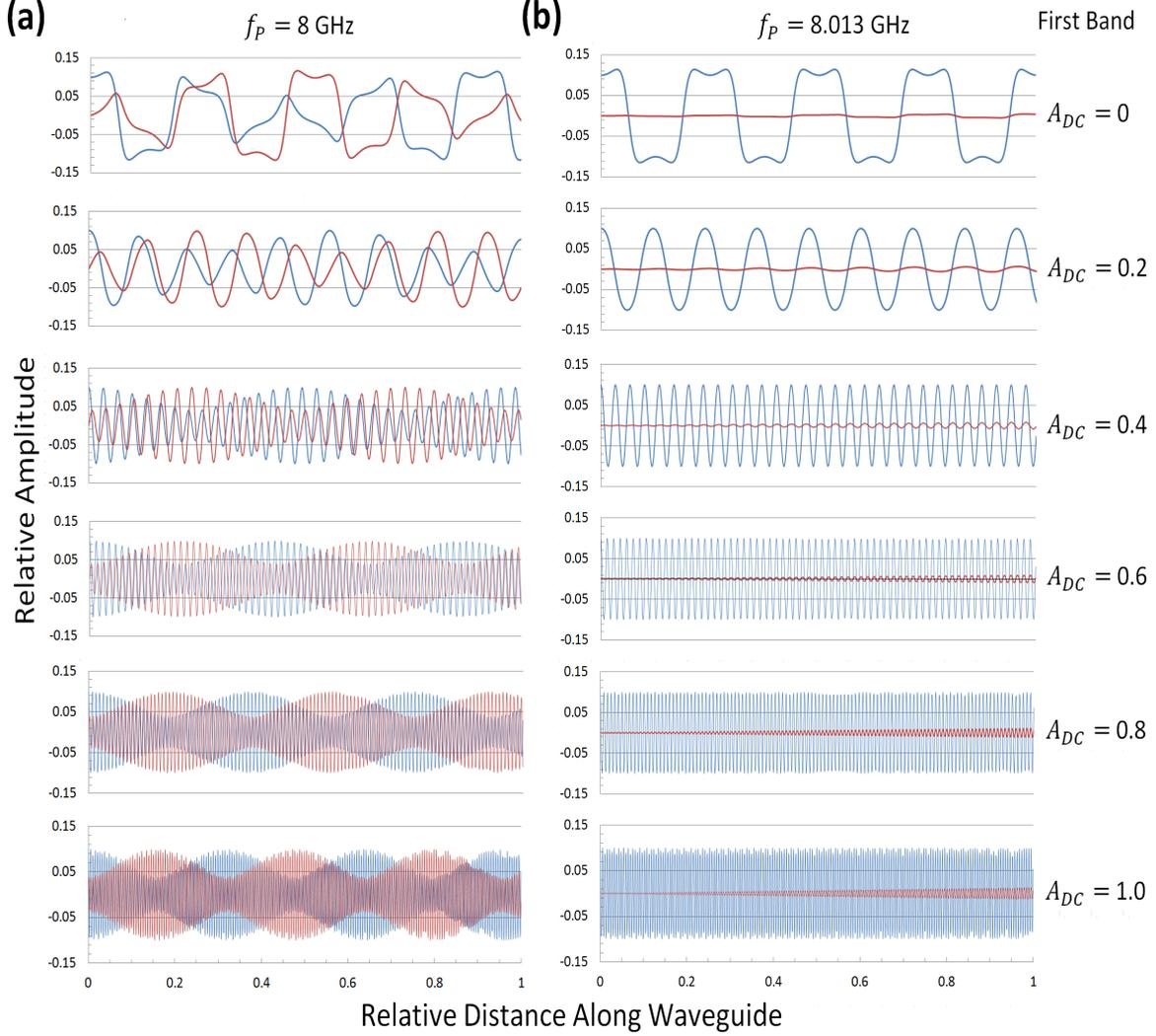
FIG. 5. Real (blue) and imaginary (red) parts of relative amplitude  $A_0^{(P)}(x)$  of first dispersion-frequency band as a function of relative position  $x/\ell_T$  along KIT. Amplitude corresponds to pump frequencies (a)  $f_P = 8$  GHz and (b)  $f_P = 8.013$  GHz (bottom of first stop gap), for values of  $A_{DC} = I_{DC}/I_*$  from zero to unity. Waveguide length is  $\ell_T = 2.0$  m and input power is set to  $P_o = 0.01$ , i.e.,  $A_0^{(P)}(0) = 0.1$ .
