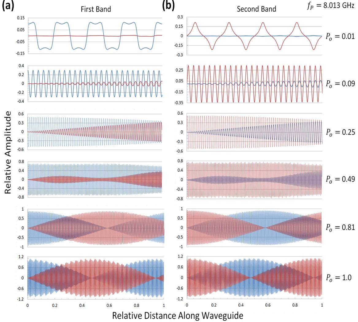
FIG. 6. Real (blue) and imaginary (red) parts of relative amplitude correspond to (a) first band,  $A_0^{(P)}(x)$ , and (b) second band,  $A_{-1}^{(P)}(x)$ , as a function of relative distance  $x/\ell_T$  along KIT, for incremented values of RF input power  $P_o$ . Waveguide length is  $\ell_T = 2.0$  m, pump frequency is  $f_P = 8.013$  GHz, at bottom of first stop gap, and no DC bias is applied.
