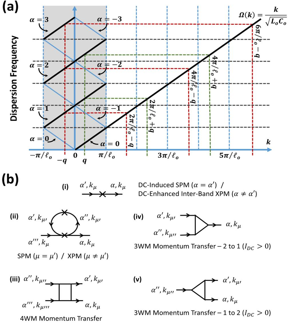
FIG. 3. (a) Comparison of reduced-zone scheme ( $-\pi/\ell_o < k < \pi/\ell_o$ ) and extended-zone scheme ( $-\infty < k < \infty$ ) representations of KIT dispersion frequencies, as described in the text. (b) The five types of multichannel parametric scattering associated with multiwave mixing within the KIT amplifier, also discussed in the text.
