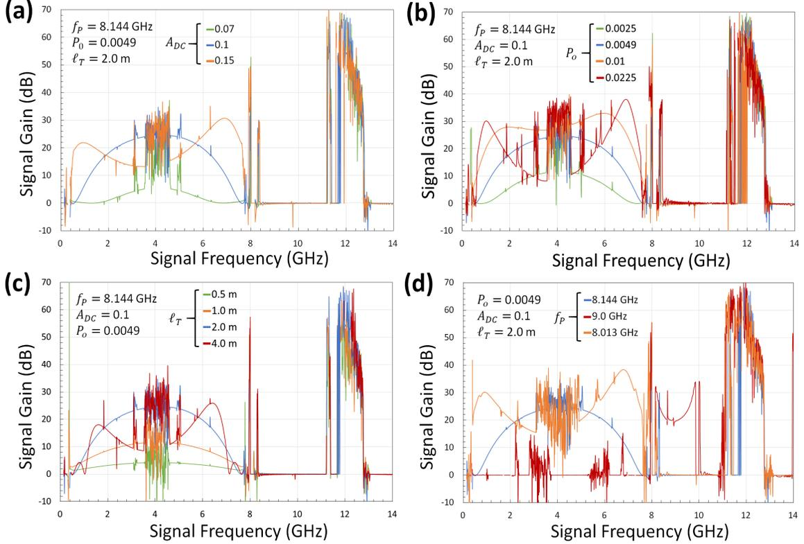
FIG. 9. Calculations of 3WM signal gain for the loading design of Table II, as described in the text, as a function of signal frequency  $f_S$ , for several values of (a) relative DC bias  $A_{DC}$ , (b) relative input power  $P_o$ , (c) waveguide length  $l_T$ , and (d) pump frequency  $f_P$ , with other parameters as labeled. In all panels optimal signal gain is the blue curve corresponding to  $A_{DC} = 0.1$ ,  $P_o = 0.0049$ ,  $l_T = 2.0$  m, and  $f_P = 8.144$  GHz.
