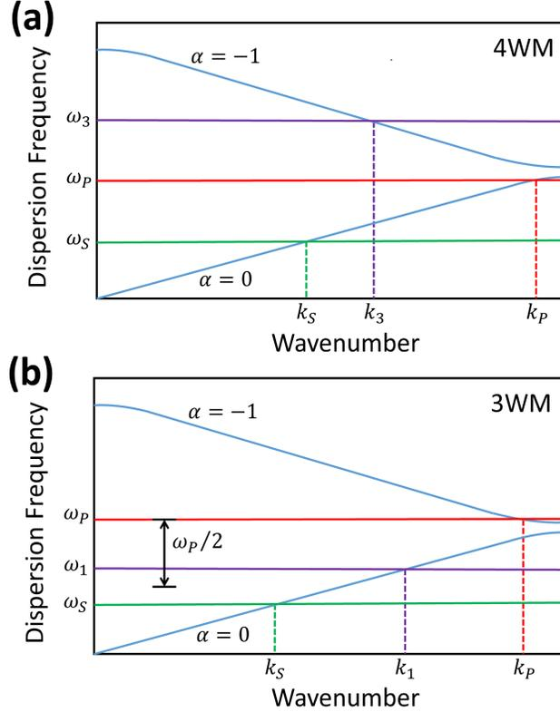
FIG. 7. Sketch showing traveling-wave pump frequency  $\omega_P$  (red) and signal frequency  $\omega_S$  (green) matched to the KIT amplifier band structure upon injection, assuming  $\omega_S < \omega_P$ . In the case of (a) the degenerate-4WM idler frequency  $\omega_3$  (purple) is shown matched to the second band ( $\alpha = -1$ ). Similarly, in (b) the idler of frequency  $\omega_1$  (purple), responsible for 3WM broadband gain, is shown matched to the first band ( $\alpha = 0$ ).
