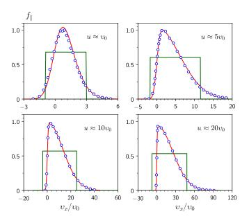
FIG. 2. The parallel IDF  $(f_{\parallel})$  for drift flows. Circles show the IDF obtained from the MC simulations. Solid lines show the IDF calculated using the model of Ref. [29] (red line) and model (3) (green line). For simplicity, all results are normalized by the maximum value of the IDF obtained from the MC simulations.
