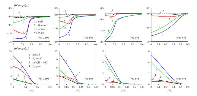
FIG. 4. Distributions of different terms in the ion momentum and energy equations (upper and lower rows, respectively). Here  $n_0 = 10^{15} \,\mathrm{m}^{-3}$ . The results are presented for the second test problem (argon,  $L = 6.7 \,\mathrm{cm}$ ) at the gas pressures 0.3, 1, 6 Pa and third test problem (helium,  $L = 6.7 \,\mathrm{cm}$ ) at the gas pressure of 4 Pa.
