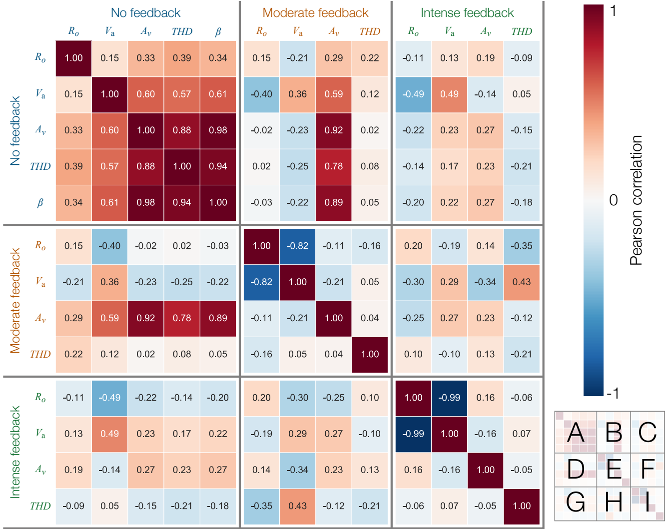
FIG. 19. Pairwise Pearson correlation values between all device and circuit properties measured in the experiments. Each block of the matrix corresponds to a combination of feedback conditions (absent, moderate or intense). These blocks are named according to the legend shown in the bottom right corner of the figure.
