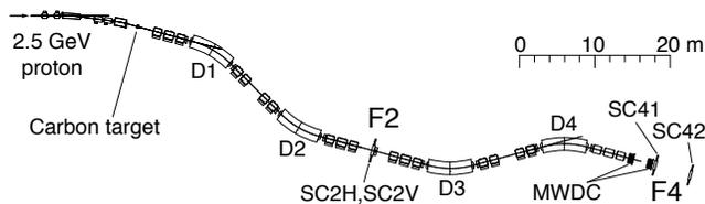
FIG. 1. A schematic view of the FRS used as a spectrometer and detectors used in the present analysis. A 2.5 GeV proton beam impinged on a carbon target. Deuterons emitted in the  $^{12}\text{C}(p, d)$  reaction were momentum-analyzed at F4 and the tracks were measured by MWDCs. Sets of 5 mm-thick plastic scintillation counters (SC2H, 2V, and SC41) and 20 mm-thick one (SC42) were installed at F2 and F4 for TOF measurement.
