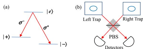
FIG. 8: Experiment principle for generating hyperentangled states between atomic ions [24]. (a) Internal energy levels of ion. The  $|+\rangle$  and  $|-\rangle$  are ground states and  $|e\rangle$  is the excited state.  $\sigma^+$  and  $\sigma^-$  are the polarized photons emitted due to the energy decay. (b) The setup of generating spin entanglement between two atomic ions confined in separated Paul traps.
