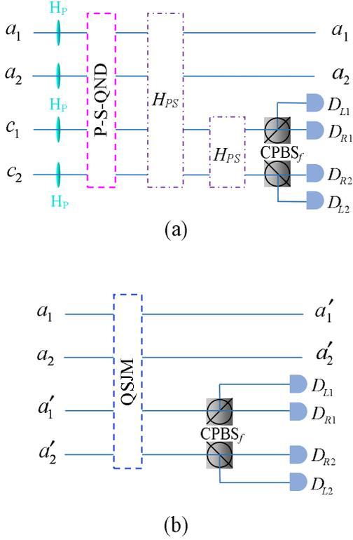
FIG. 22: (a) Schematic diagram of the first step of the two-step hyper-EPP with the P-S-QND [51]. The operations performed on the photons  $B$  and  $D$  are the same as the ones performed on the photons  $A$  and  $C$ . (b) Schematic diagram of the second step of the two-step hyper-EPP with QSJM. The operations performed on the photons  $B$  and  $B'$  are the same as the ones performed on the photons  $A$  and  $A'$ .
