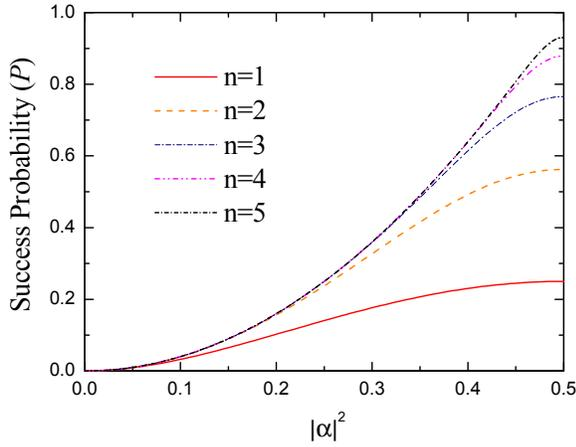
FIG. 17: Success probability of the hyper-ECP for a pair of partially hyperentangled Bell states under the iteration numbers ( $n$ ) [44, 48]. The parameters of the polarization-spatial partially hyperentangled Bell state are chosen as  $|\alpha| = |\gamma|$  and  $|\beta| = |\delta|$ .
