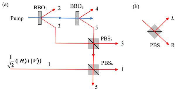
FIG. 7: Experiment setup for generating ten-qubit five-photon hyperentangled state [22]. (a) Generation of five-photon polarization entangled state with postselection. (b) Creation of polarization-spatial mode entanglement with PBS.  $L$  and  $R$  are two different spatial modes.
