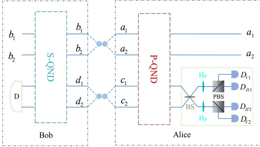
FIG. 16: Schematic diagram of the polarization-spatial hyper-ECP for unknown partially hyperentangled Bell states [45, 48], resorting to the Schmidt projection method. D represents the same operations as the ones performed by Alice in the green dotted box.
