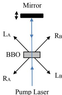
FIG. 4: Schematic diagram of the setup to generate hyperentanglement in both polarization and spatial-mode DOFs.
