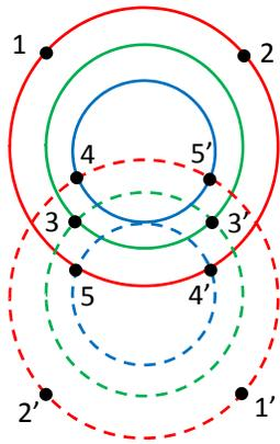
FIG. 3: Schematic diagram of the type-II phase-matching curves. The upper half (solid lines) are three extraordinary-polarized cones with different wavelengths. The ordinary-polarized cones are shown in the lower half (dashed lines) with corresponding wavelength. The numbered points represent the areas of directions to extract hyperentangled states.
