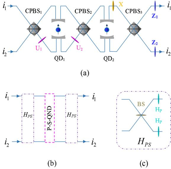
FIG. 21: (a) Schematic diagram of the polarization-spatial phase-check QND (P-S-QND) [51].  $Z_i$  ( $i = 1, 2$ ) represents a wave plate which is used to perform a polarization phase-flip operation  $\sigma_z^P = -|R\rangle\langle R| + |L\rangle\langle L|$  on a photon. (b) Schematic diagram of the polarization-spatial parity-check QND. (c) Schematic diagram of  $H_{PS}$  which is used to perform the Hadamard operations on both the polarization and spatial-mode DOFs of a photon.
