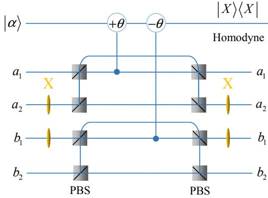
FIG. 15: Schematic diagram of the polarization parity-check quantum nondemolition detector (P-QND) with the cross-Kerr nonlinearity [48].
