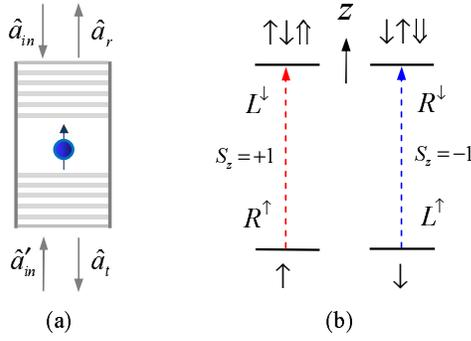
FIG. 19: (a) A double-sided QD-cavity system. (b) The spin-dependent optical transitions of a negatively charged exciton  $X^-$  with circularly polarized photons [51].  $L^\uparrow$  ( $L^\downarrow$ ) and  $R^\uparrow$  ( $R^\downarrow$ ) represent the left and the right circularly polarized lights with their input directions parallel (antiparallel) with  $z$  direction, respectively.
