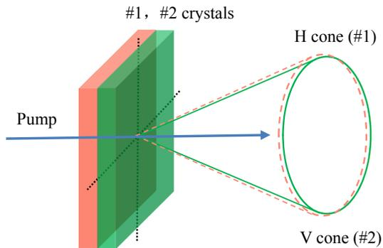
FIG. 1: Type-I polarization entanglement sources.
