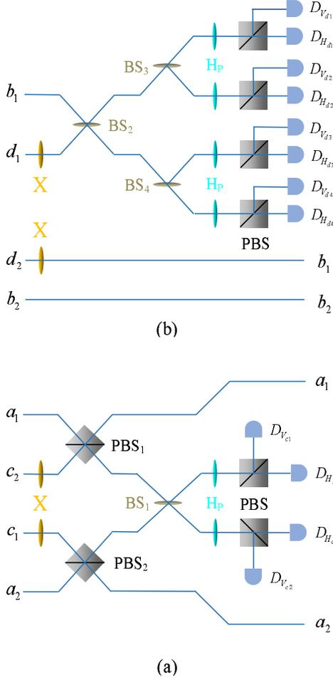
FIG. 14: Schematic diagram of the polarization-spatial hyper-ECP for partially hyperentangled Bell states with unknown parameters [43], resorting to the Schmidt projection method. (a) Operations performed by Alice. (b) Operations performed by Bob. X represents a half-wave plate which is used to perform a polarization bit-flip operation  $\sigma_x^P = |H\rangle\langle V| + |V\rangle\langle H|$ .
