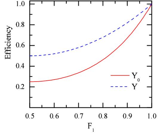
FIG. 24: The efficiency of the two-step hyper-EPP for mixed hyperentangled Bell states [51].  $Y_0$  ( $Y$ ) is the efficiency of the first round of the hyper-EPP process without (with) QSJM. The parameters of the initial mixed hyperentangled Bell state are  $F_1 = F_2$ .
