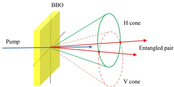
FIG. 2: Non-collinear type-II phase-matching spontaneous parametric down-conversion process.
