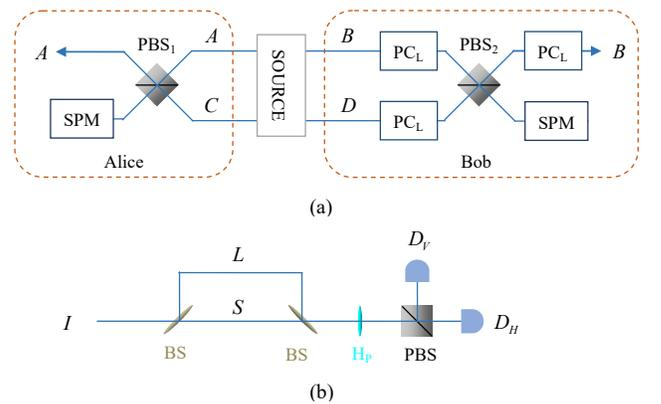
FIG. 18: (a) Schematic diagram of the polarization-time-bin hyper-ECP for partially hyperentangled Bell states with unknown parameters [49], resorting to the Schmidt projection method.  $PC_L$  ( $PC_S$ ) represents a Pockels cell, which is used to perform polarization bit-flip operation on the  $L$  ( $S$ ) component. (b) Schematic diagram of a single-photon measurement (SPM).
