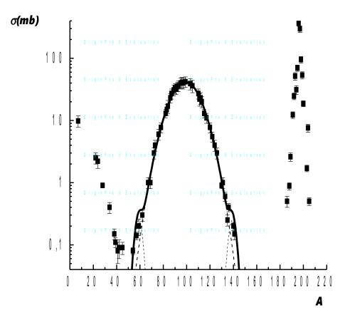
FIG. 1. Mass-yield distribution for the interaction of  $^{197}$ Au with 137.5 MeV  $^{11}$ B ions. The dashed curves corresponds to the isobaric symmetric and asymmetric fission cross sections as a function of the mass of the fragments A. The black continuous curve corresponds to the total mass-yield, and experimental data are represented by the solid squares.
