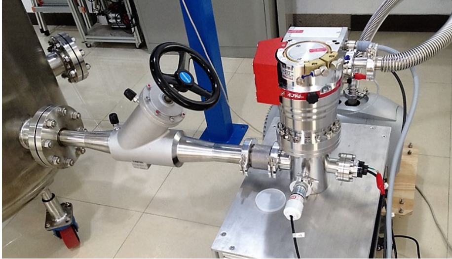
Figure 16: The High pressure valve (model number: HFC2003-10PC2FSM from Carten-Fujikin), turbo-pump(HiPace300 from Pfeiffer), fore-pump (PTS300 from Agilent) and vacuum gauges connected to our prototype TPC.
