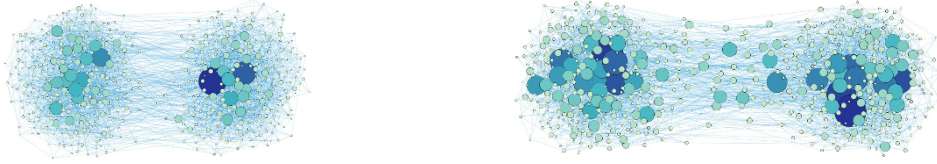
Figure 12 – (left) BA communities interconnected by scale-free links (no inter-community assortativity); (right) BA communities interconnected by scale-free links (with inter-community assortativity). In both cases, N = 600 , \rho = 0.1 , the size of each node is proportional to its overall degree and the spatial position of nodes represents the equilibrium configuration of the Force Atlas visualization algorithm [50].
