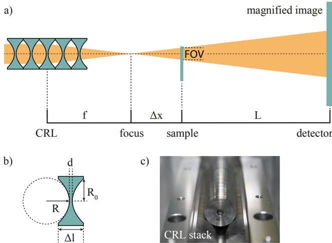
FIG. 3. a) Schematic of the Be CRL setup in PCI geometry. The lens stack has a focal length  $f$ . The focus is placed at a distance  $\Delta x$  in front of the sample. A detector is then positioned a distance  $L$  after the sample, leading to a magnification  $M = (L + \Delta x)/\Delta x$ . b) Sketch of a single parabolic Be CRL indicating relevant geometric parameters. c) Image of a stack of Be CRLs aligned in a lens holder.
