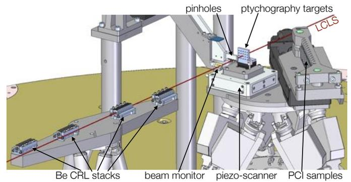
FIG. 4. Ptychographic sample environment. A sample with nanometer sized structures is positioned close to the x-ray focus and normal to the beam. It is located on a 3-axis piezo-drive stage (PI P-733) that can scan the sample through the beam with a nm repeatability and sub-nanometer resolution. Pinholes of varying sizes can be placed in front of the target.
