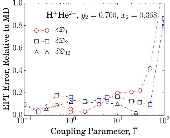
FIG. 5. Errors in EPT diffusion coefficients, relative to MD values for a 70% helium (by mass)  $\text{H}^+\text{He}^{2+}$  BIM. Red circles: hydrogen self-diffusion coefficient. Blue squares: helium self-diffusion coefficient. Black triangles: interdiffusion coefficient. Dashed lines are included to guide the eye.
