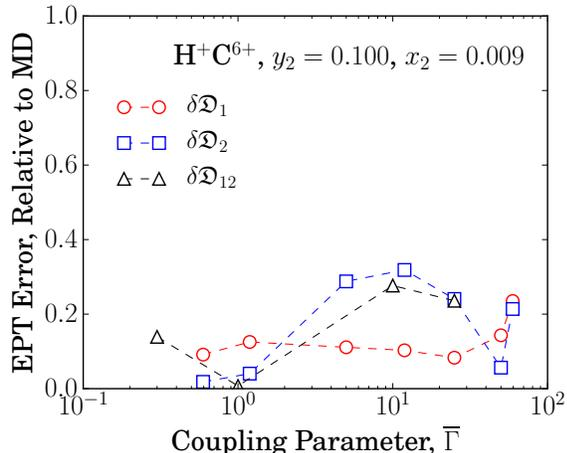
FIG. 9. Errors in EPT diffusion coefficients, relative to MD values for a 10% carbon (by mass)  $\text{H}^+\text{C}^{6+}$ BIM. Red circles: hydrogen self-diffusion coefficient. Blue squares: carbon self-diffusion coefficient. Black triangles: interdiffusion coefficient. Dashed lines are included to guide the eye.
