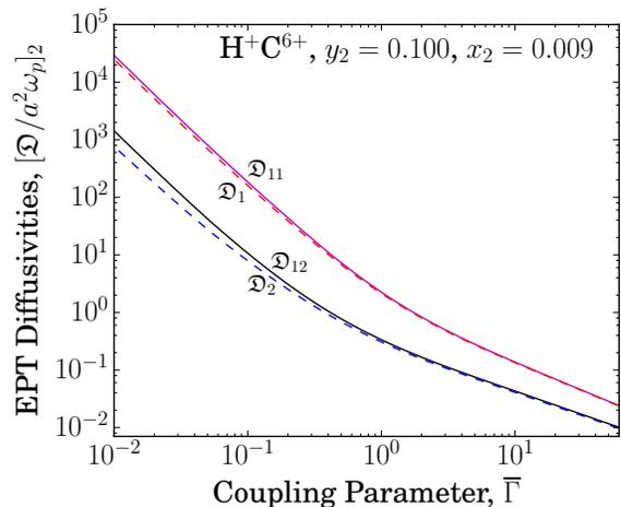
FIG. 10. Test of the impurity-limit approximations Eqs. (43)-(44) in a 0.9% (by mole)  $\text{H}^+\text{C}^{6+}$ BIM. All diffusion coefficients plotted are second-order EPT results.
