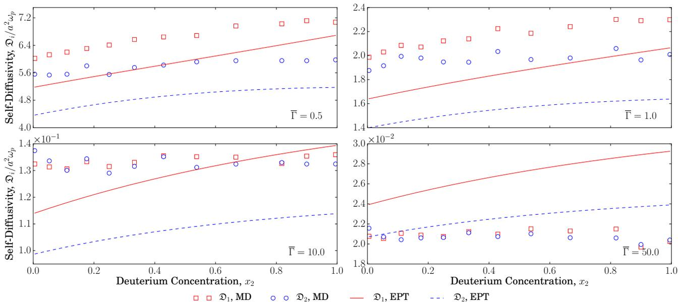
FIG. 7. Dependence of the diffusion coefficients on deuterium mole fraction at selected coupling strengths for a  $\text{H}^+\text{D}^+$  BIM. Lines are EPT predictions for  $\mathfrak{D}_1$  (solid red) and  $\mathfrak{D}_2$  (dashed blue). Shapes are MD results.
