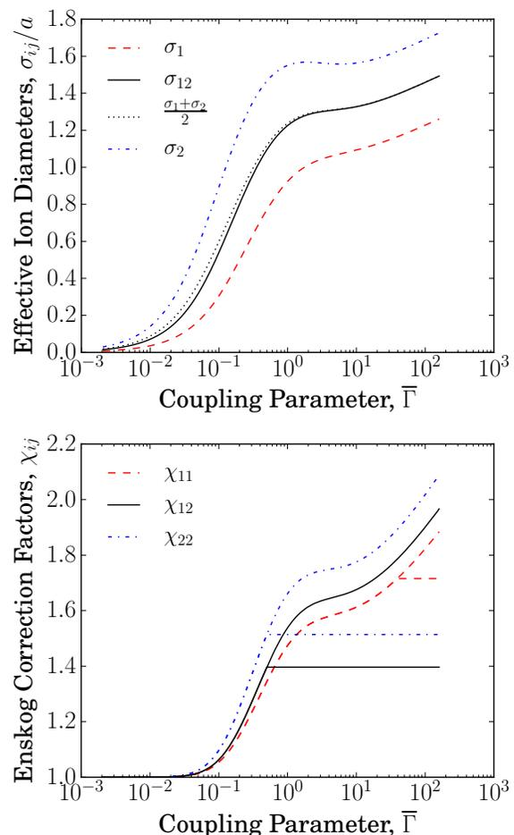
FIG. 2. (a) Effective ion diameters and (b) modified Enskog correction factors (with and without virial cutoff) in a 36.8% helium (by mole)  $\text{H}^+\text{He}^{2+}$ BIM.
