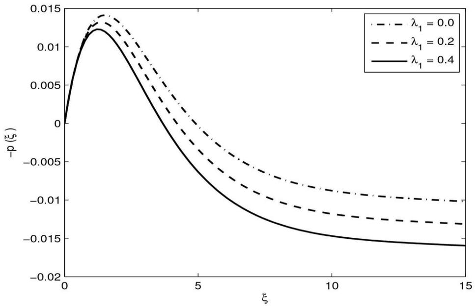
Fig. 9: The influence of radial slip on pressure distribution in the presence of tangential slip
