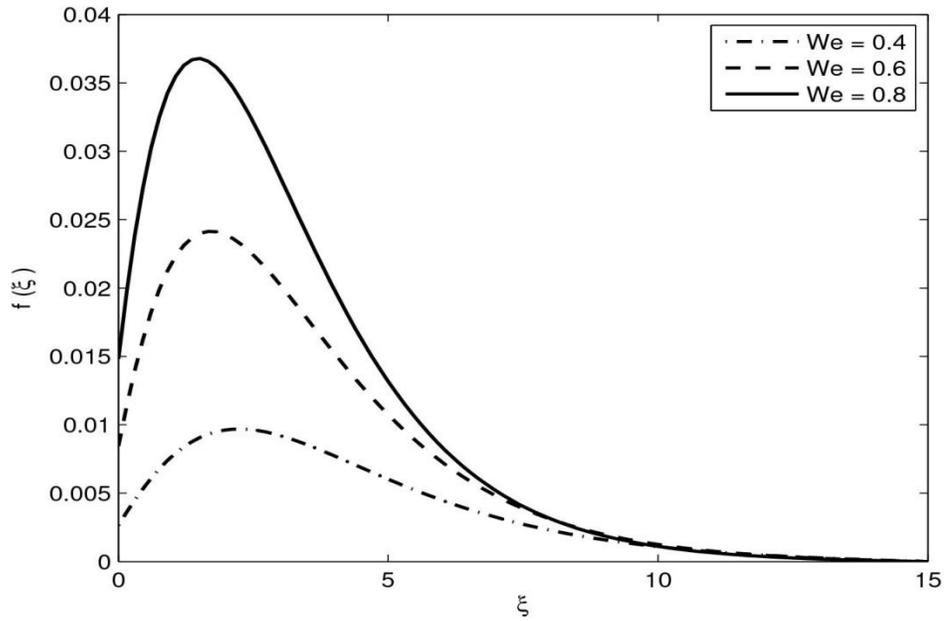
Fig. 2: The influence of Weissenberg number on radial velocity in the presence of anisotropic slip
