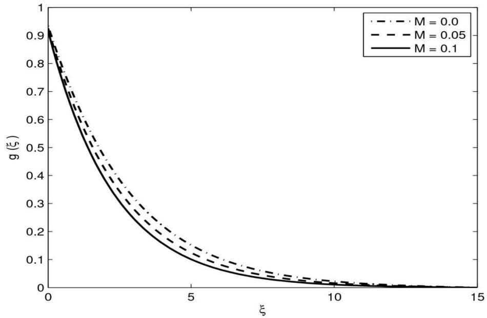
Fig. 16: The influence of magnetic field on tangential velocity profile in the presence of anisotropic slip
