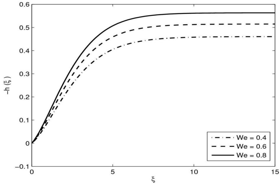
Fig. 4: The influence of Weissenberg number on axial velocity in the presence of anisotropic slip
