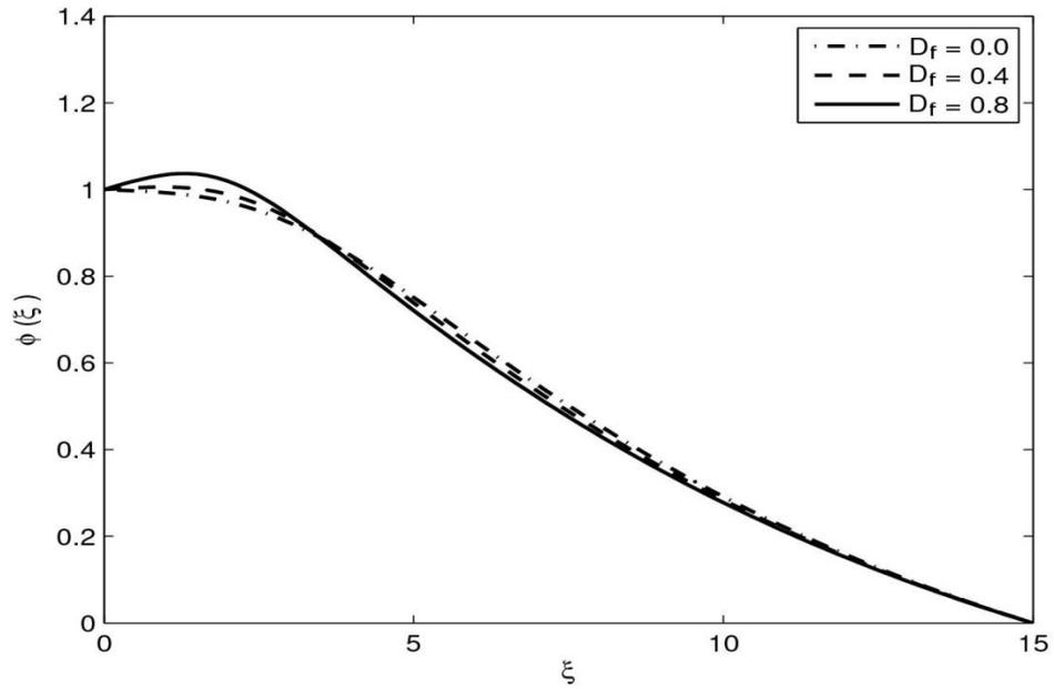
Fig. 20: The influence of Dufour parameter on concentration distribution in the presence of anisotropic slip
