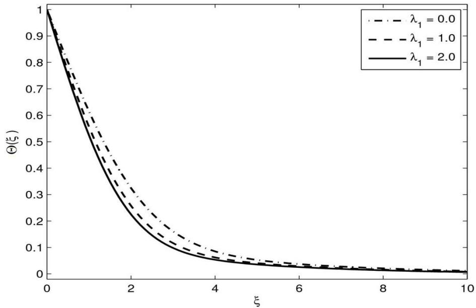
Fig. 10: The influence of radial slip on temperature distribution in the presence of tangential slip
