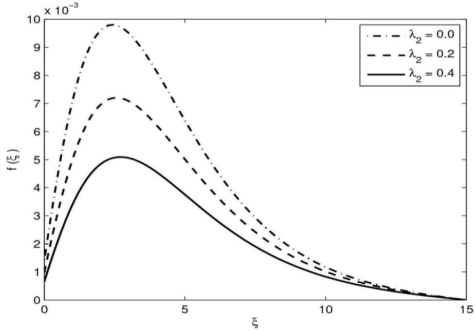
Fig. 12: The influence of tangential slip on radial velocity profile in the presence of radial slip
