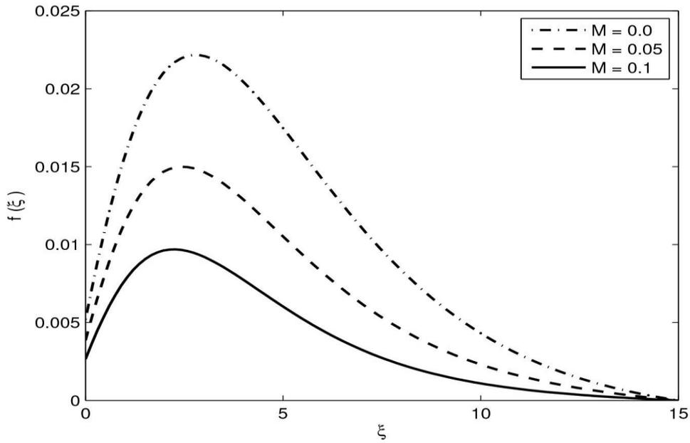
Fig. 15: The influence of magnetic field on radial velocity profile in the presence of anisotropic slip
