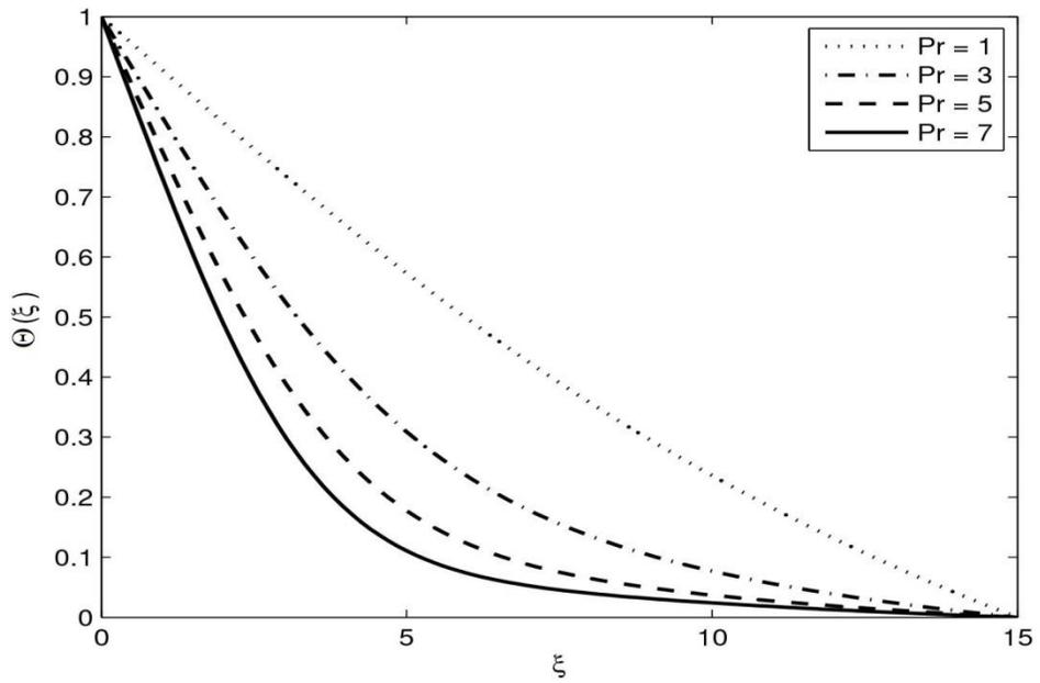
Fig. 21: The influence of Prandtl number on temperature distribution in the presence of anisotropic slip
