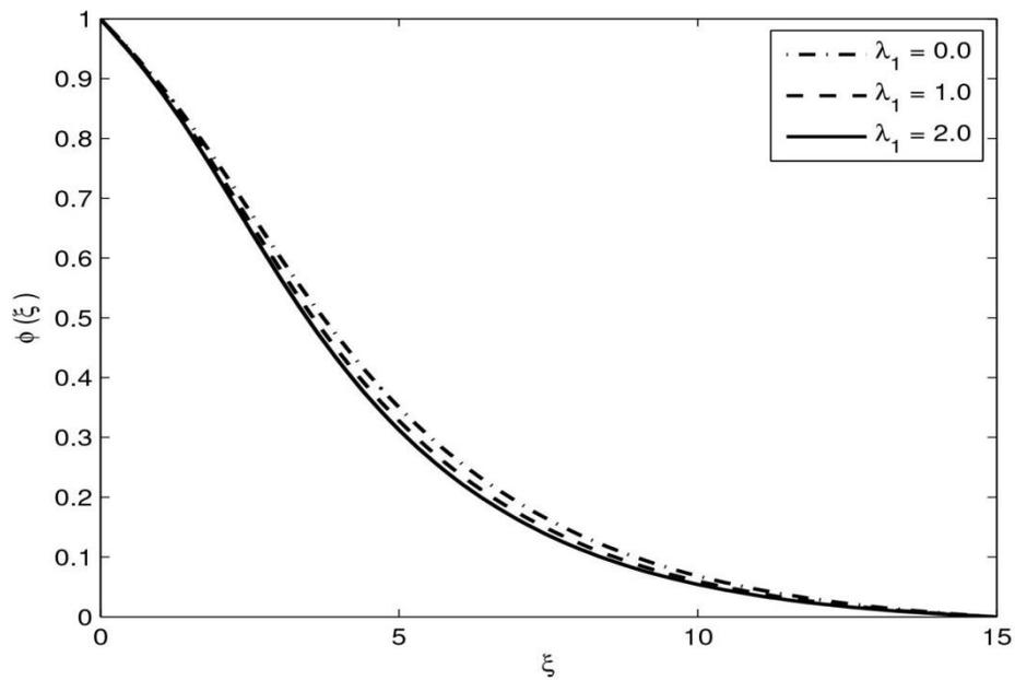
Fig. 11: The influence of radial slip on concentration distribution in the presence of tangential slip
