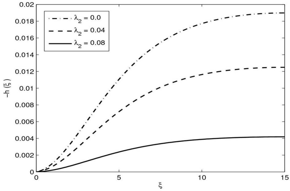
Fig. 14: The influence of tangential slip on axial velocity profile in the presence of radial slip
