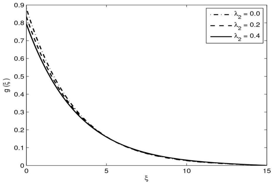
Fig. 13: The influence of tangential slip on tangential velocity profile in the presence of radial slip
