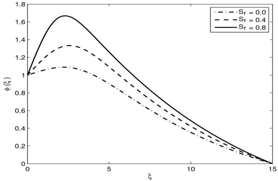
Fig. 18: The influence of Soret parameter on concentration distribution in the presence of anisotropic slip
