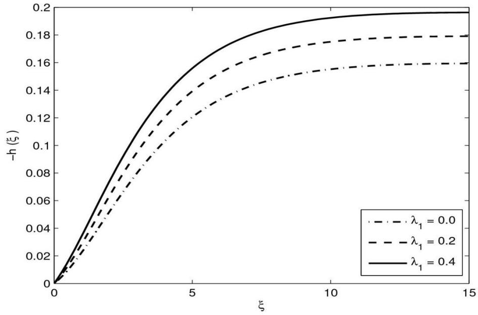
Fig. 8: The influence of radial slip on axial velocity in the presence of tangential slip
