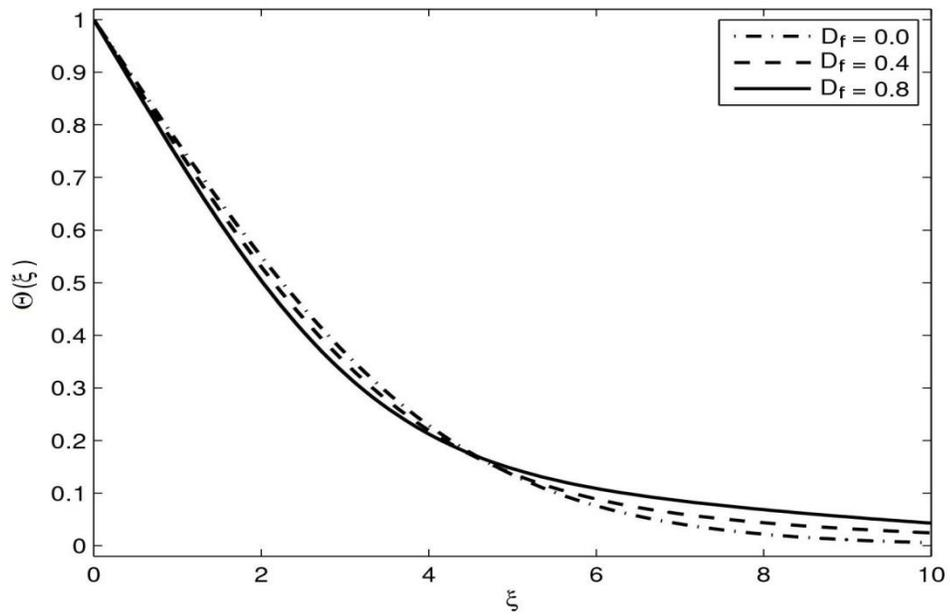
Fig. 19: The influence of Dufour parameter on temperature distribution in the presence of anisotropic slip
