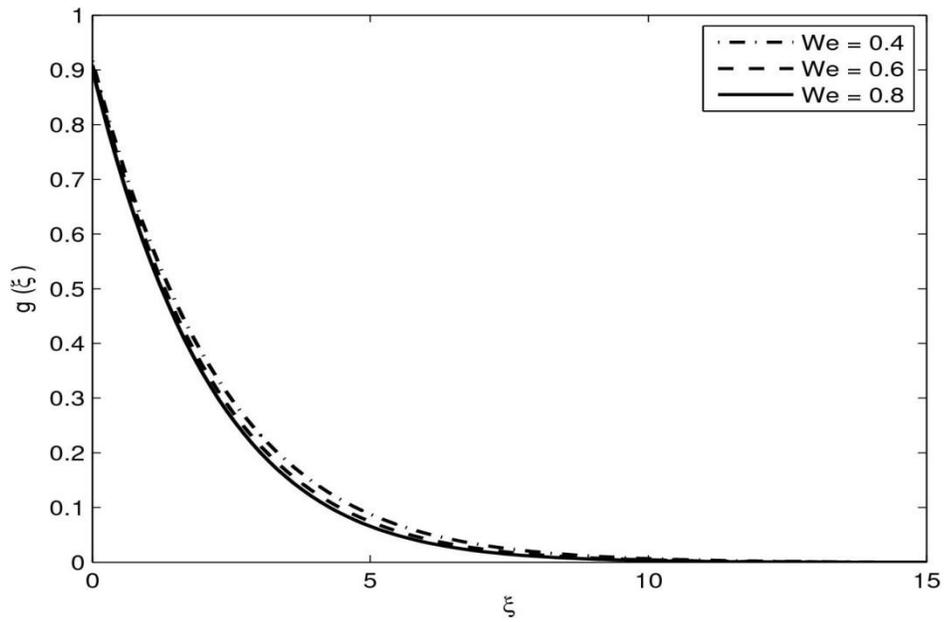
Fig. 3: The influence of Weissenberg number on tangential velocity in the presence of anisotropic slip
