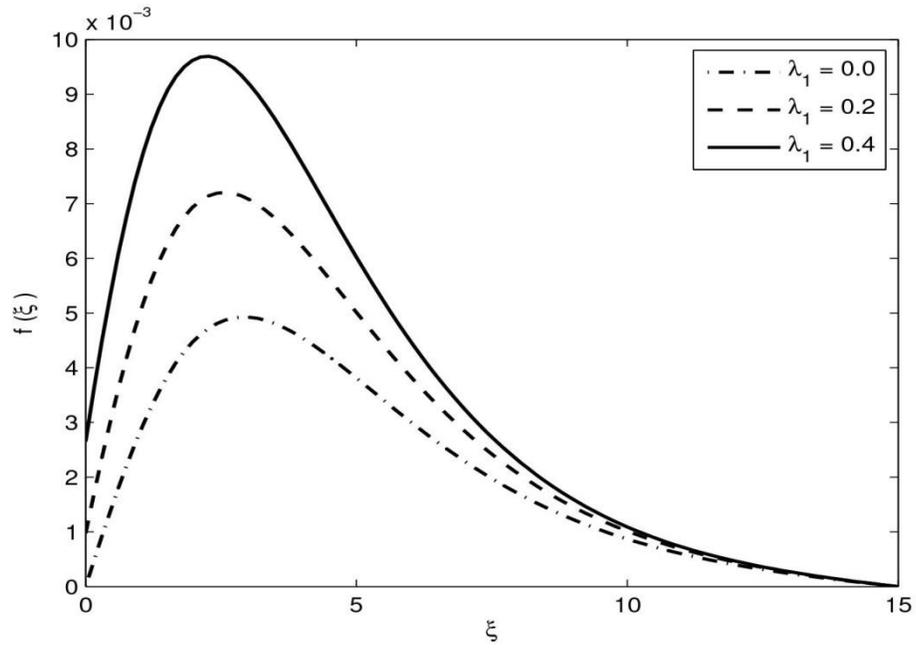
Fig. 6: The influence of radial slip on radial velocity in the presence of tangential slip
