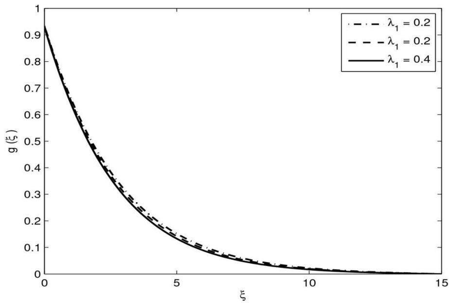
Fig. 7: The influence of radial slip on tangential velocity in the presence of tangential slip
