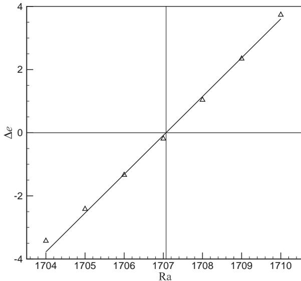
FIG. 5: Total internal energy increment  $\Delta e (\times 10^{-10})$  changes with different Rayleigh numbers. Triangles are the numerical results; the solid line is the linear fit for the simulations. The critical Rayleigh number extrapolated is  $\text{Ra}_c = 1707.07$ .
