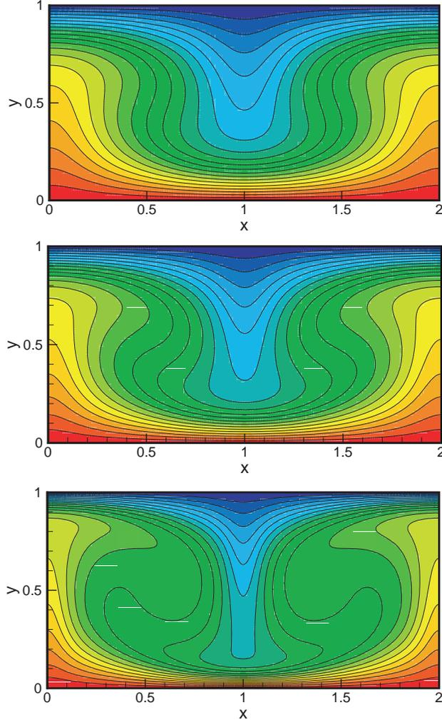
FIG. 6: The normalized temperature  $(T - T_0)/\Delta T$  distribution for Rayleigh-Bénard convection flow. From top to bottom:  $Ra=5000$ ,  $10000$  and  $50000$ . A total of 19 equidistant lines are plotted.
