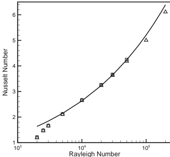
FIG. 7: Nusselt number vs Rayleigh number. Triangles: the present thermal CLBM; squares: reference data from Ref. [39]; and solid line: the empirical formula  $Nu = 1.56(Ra/Ra_c)^{0.256}$ .
