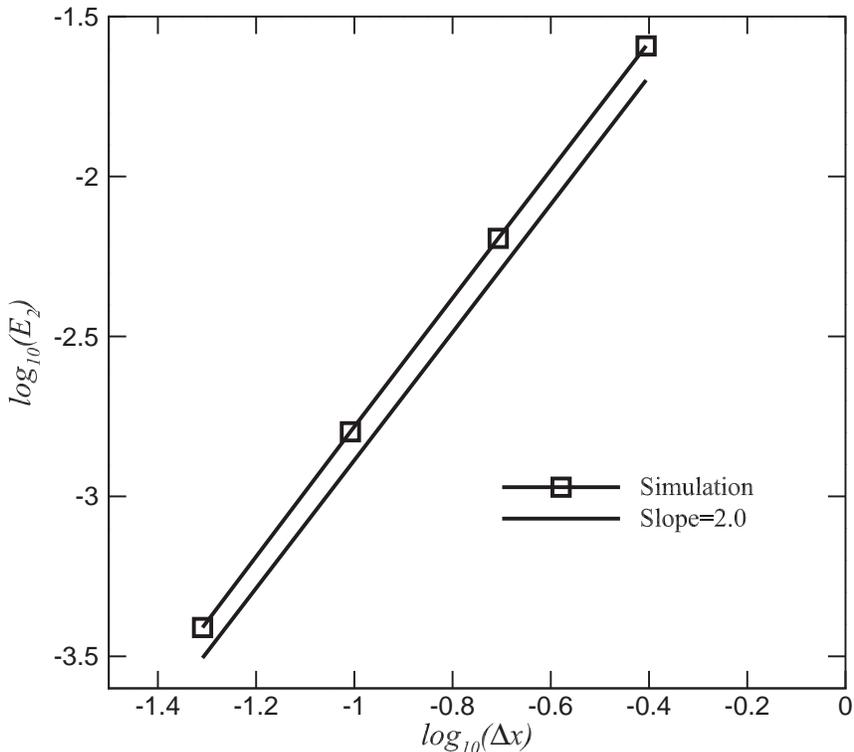
FIG. 2: Relative error  $E_2$  at different space step at  $Re=20$ .
