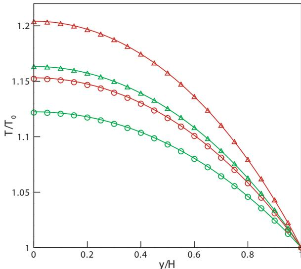
FIG. 3: Comparison between the simulation (symbols) and analytical (solid lines) results for dimensionless temperature profiles at  $\text{Ma} = 0.35$ , with  $\text{Pr}=5$  (red ones) and 4 (green ones). Deltas and circles are the simulation results for  $\gamma = 5/3(b = 3)$  and  $3/2(b = 4)$ , respectively.
