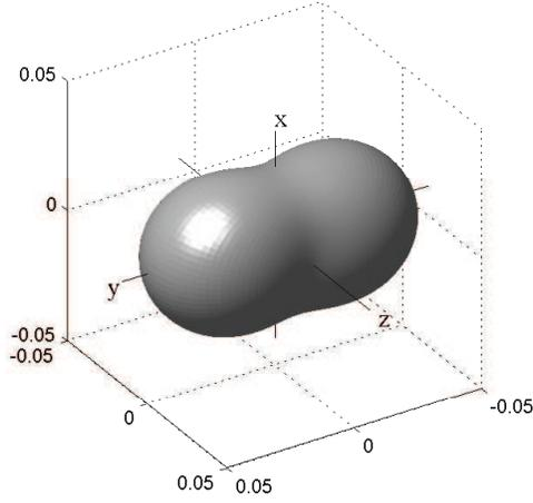
Figure 2: The angular dependence of DR intensity as direction diagram for the passage of the real charge under  $b = R$  (sliding incidence on the sphere, when DR intensity is maximal for the whole range of wavelengths) and  $R\omega/v_0 = 2.34$  (this choice is due to the maximum of DR spectrum (see below) falls on  $b\omega/v_0 \approx 2.34$  and  $b = R$  in the given case).
