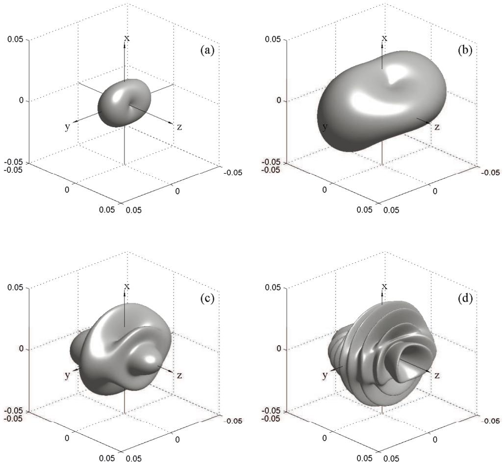
Figure 5: Direction diagrams of the radiation emitted under incidence of the real charge under  $b = R/\sqrt{2}$  for  $v_0 = 0.1c$ ,  $R\omega/v_0 = 1, 10, 50, 200$ .
