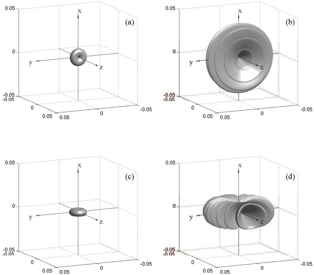
Figure 6: Direction diagrams of the partial contributions to the radiation emitted under incidence of the real charge under  $b = R/\sqrt{2}$  for  $R\omega/v_0 = 200$ ,  $v_0 = 0.1c$ .
