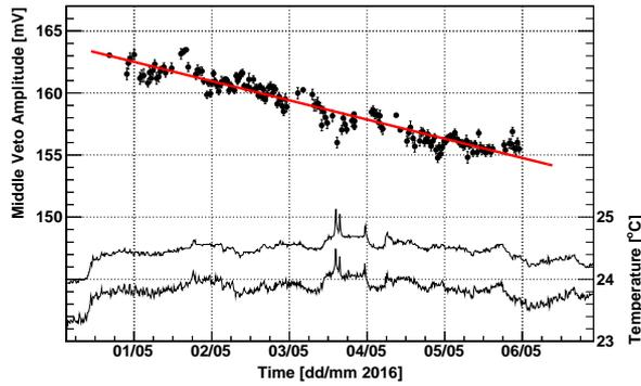
Figure 10: In-beam aging of a 1mm thick BC-404 plastic scintillator. The points show the mean amplitudes obtained for the beam particles ( $^{108}\text{Sn}$  and  $^{112}\text{Sn}$  at 300 AMeV). The line shows a linear fit to the points. The histograms show the local temperature variation at the top (upper histogram) and at the bottom (lower one) of the middle Veto paddle.
