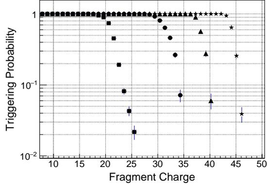
Figure 9: Measured efficiency of a thin VETO paddle. Different symbols (squares, points, triangles and stars) correspond to increasing thresholds applied to the VETO signal amplitude.
