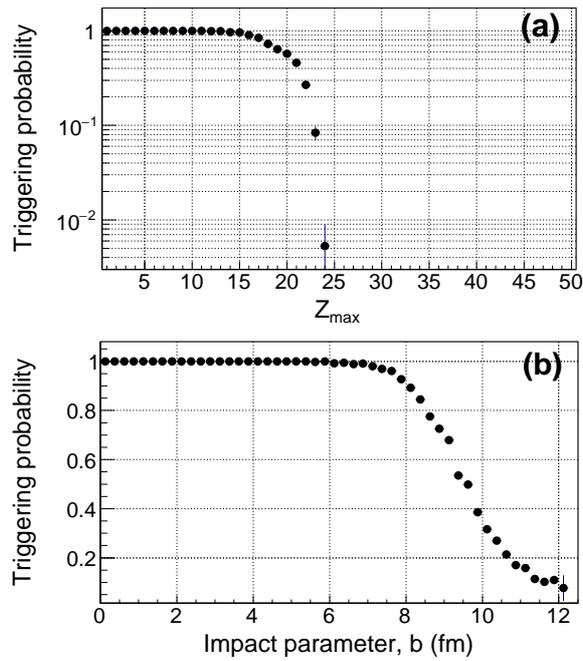
Figure 2: Simulated trigger efficiency of the KATANA detector: a) acceptance for the charged fragments hitting the VETO paddles; b) distribution of the accepted impact parameters.
