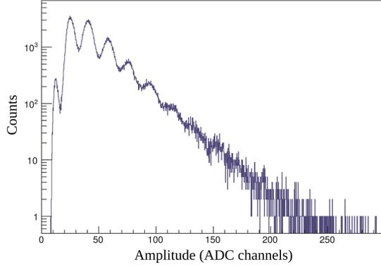
Figure 6: Single-photon amplitude resolution achieved for thick paddles equipped with S12572-025P elements.
