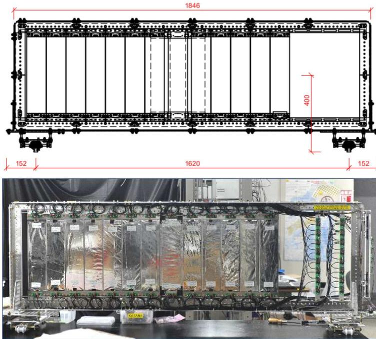
Figure 3: Top panel: a technical drawing of the KATANA detector with the external dimensions in mm. Bottom panel: a photo of the detector before mounting it inside the SAMURAI vacuum chamber.
