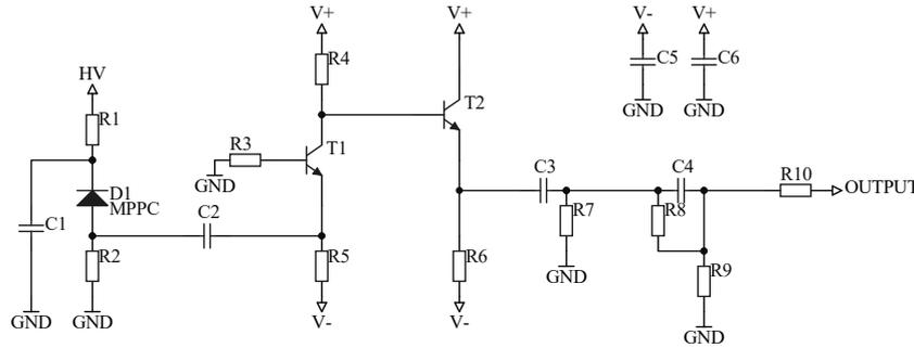
Figure 5: Schematic of the preamplifier for MPPC.
