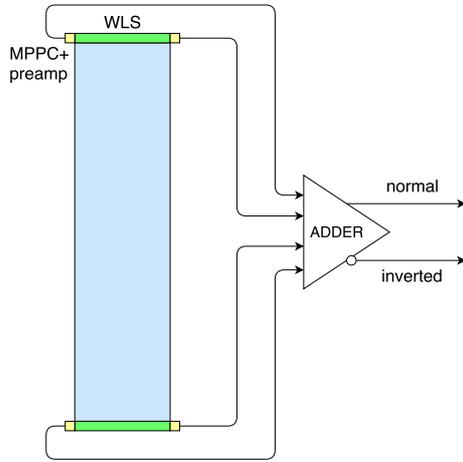
Figure 1: Schematic view of a VETO paddle
