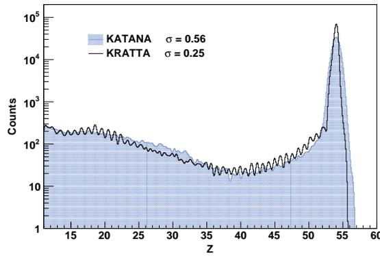
Figure 8: Charge resolution obtained at HIMAC with the KATANA prototype plastic bar (hatched histogram) and with the KRATTA module (black line) for the  $^{132}\text{Xe}$  fragmentation at 300 AMeV. Note the single charge resolution for the KRATTA detector.
