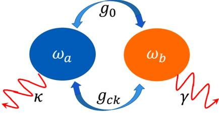
FIG. 1. (Color online) Schematic diagram of the considered optomechanical system. An optical mode (with frequency  $\omega_a$ ) couples the mechanical mode (with frequency  $\omega_b$ ) via the radiation-pressure coupling  $g_0$  and an additional cross-Kerr coupling  $g_{ck}$ . Here,  $\kappa$  is the optical decay rate and  $\gamma$  is the mechanical damping rate.
