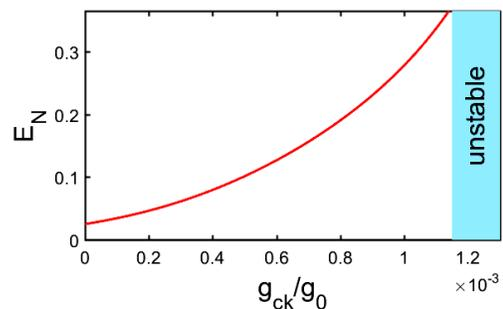
FIG. 3. (Color online)  $E_N$  as a function of the normalized cross-Kerr coupling strength  $g_{ck}/g_0$ , at a fixed  $P/P_0 = 2.0$ ,  $\Delta_0/\omega_b = 0.5$  and  $\kappa/\omega_b = 0.4$ .
