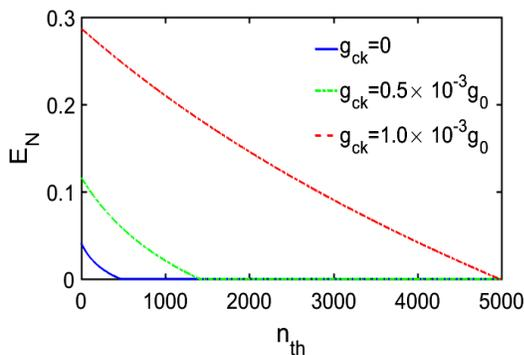
FIG. 6. (Color online)  $E_N$  versus the mean thermal phonon number for different cross-Kerr coupling strengths. The other parameters are fixed at  $\Delta_0/\omega_b = 0.5$ ,  $\kappa/\omega_b = 0.4$  and  $P/P_0 = 2.0$ .
