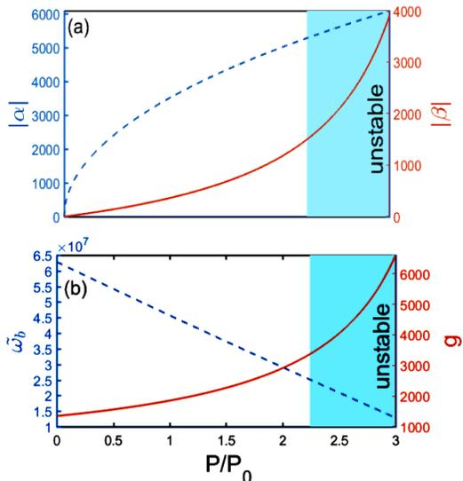
FIG. 2. (Color online) (a) The steady-state amplitudes  $|\alpha|$  (blue dashed) and  $|\beta|$  (red solid), and, (b) the modified mechanical frequency  $\tilde{\omega}_b$  (blue dashed) and coupling strength  $g$  (red solid) versus the driving power  $P/P_0$ . The shaded (cyan) region corresponds to the unstable phase of the optomechanical system. The other parameters are fixed at:  $g_{ck} = 10^{-3}g_0$ ,  $\kappa/\omega_b = 0.4$  and  $\Delta_0/\omega_b = 0.5$ .
