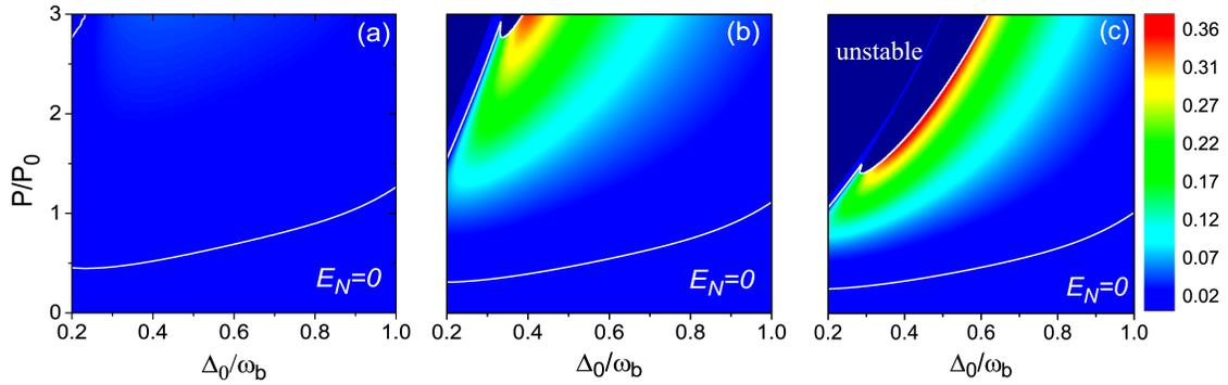
FIG. 4. (Color online) Contour plot of  $E_N$  versus the normalized detuning  $\Delta_0/\omega_b$  and driving power  $P/P_0$ , for  $g_{ck} = 0$  (a) (no cross-Kerr coupling),  $g_{ck} = 0.5 \times 10^{-3}g_0$  (b), and  $g_{ck} = 1.0 \times 10^{-3}g_0$  (c). The optical decay rate is fixed at  $\kappa/\omega_b = 0.4$ .
