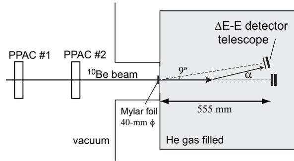
Fig. 2. The experimental setup for the resonant scattering measurement.
