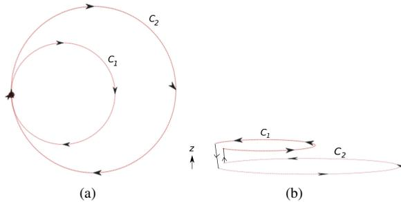
**Figure 7.** (a) A double winding loop, which runs once around contour  $C_1$ , and once around the coplanar loop  $C_2$ . (b) A “shifted” double winding loop, in which contours  $C_1$  and  $C_2$  lie in planes parallel to the  $x-y$  plane, but are displaced from one another in the transverse direction by distance  $\delta z$ , and are connected by lines running parallel to the  $z$ -axis.
