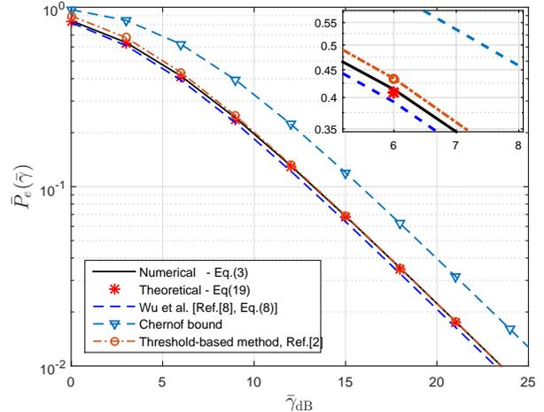
Fig. 3. A comparison of different approximation techniques: average PER of BPSK modulation in Rayleigh block-fading with  $N = 32$ .
