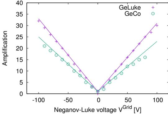
Figure 2: Amplification as a function of the applied voltage achieved by Neganov-Luke effect with the GeLuke and GeCo light detectors. The measurement was performed at 18 mK and light pulses were generated by a 820 nm LED excited with 5  $\mu$ s-width voltage square pulses. The GeCo detector develops parasitic currents above 50 V with a consequent amplification reduction. Linear fits are shown. A slight asymmetry is observed with respect to voltage polarity.
