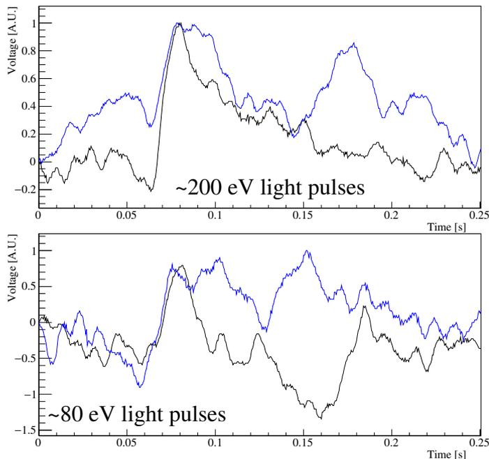
Figure 6: Typical Cherenkov light signals read out by the GeCo LD. Top: signals corresponding to  $\approx 200$  eV. Bottom: signals corresponding to  $\approx 80$  eV. The different colours simply distinguish between a pulse that can be eye-recognized (black) and a pulse that is "confused" within micro-phononic noise (blue). All signals are aligned at the maximum reconstructed amplitude of the pulse, 80 ms.
