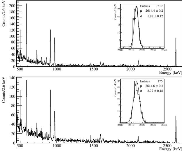
Figure 3:  $^{228}\text{Th}$  calibration spectra collected over 64 hours. Top  $^{130}\text{TeO}_2$ -1; bottom  $^{130}\text{TeO}_2$ -2. The 2615 keV  $\gamma$  peak of  $^{208}\text{Tl}$  is highlighted in the inset.
