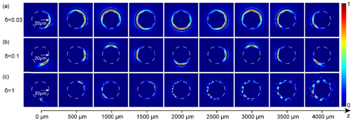
Fig.2. The cross-sectional intensity distribution of helical beams with spatial frequency width  $\delta$  set to be (a) 0.03, (b) 0.1, and (c) 1, corresponding to Fig. 1(c). The radius and period of the predesigned helical trajectory are 20 and 2000  $\mu\text{m}$ , respectively.
