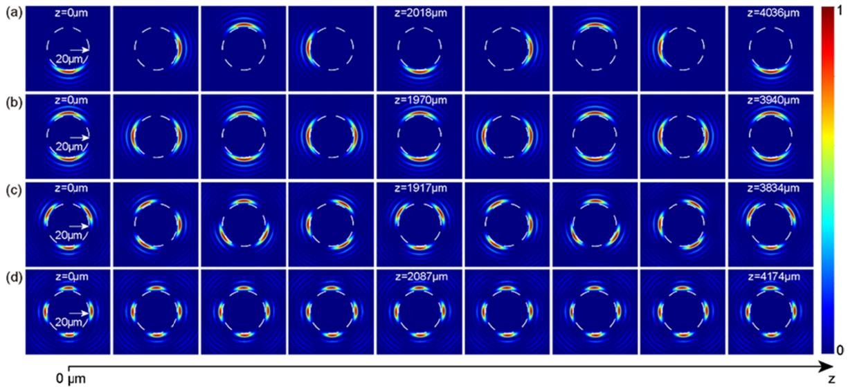
Fig.3. Propagation dynamics of helical beams with different number of main lobes. The helical beams presented includes (a) one-lobe, (b) two-lobe, (c) three-lobe, and (d) four-lobe, with slightly different period of 2018, 1970, 1917, and 2087  $\mu\text{m}$ , respectively.
