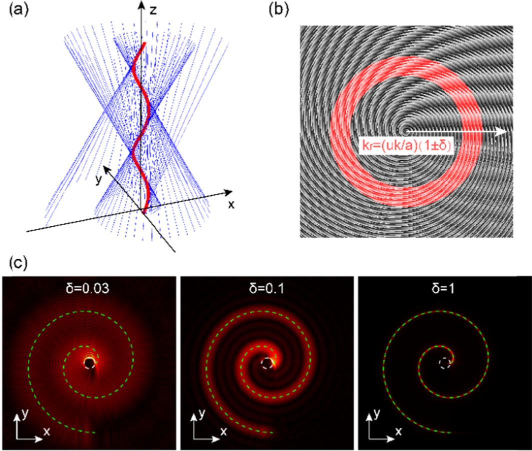
Fig. 1. Design of the helical beams. (a) Superposition of light rays in blue to form a helical caustic in red. (b) Angular spectrum of the helical beam in the initial plane, with the phase distribution in grayscale and an additional ring-shape amplitude distribution in red with a spatial frequency width described by  $\delta$ . (c) The initial field distribution corresponding to different spatial frequency width  $\delta$ .
