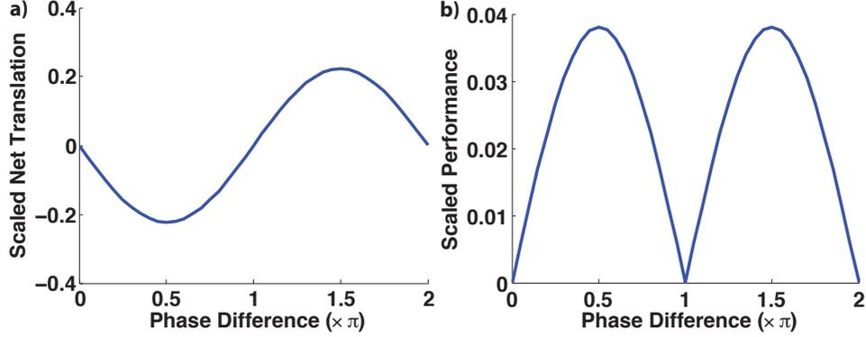
**Fig. 3.3** The scaled net translation (a) and performance (b) with respect to phase difference between the two controls  $\hat{l}$  and  $\hat{R}_1$ , with  $l_0 = 12$ , simulated by the RPY approximation.
