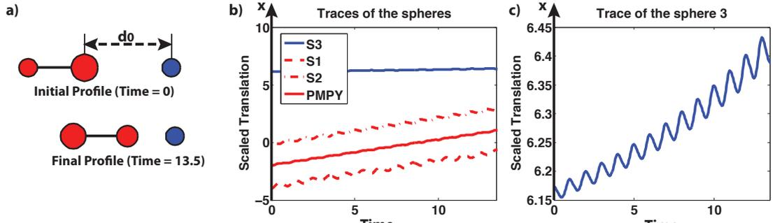
**Fig. 4.2** Simulation of a PMPY swimmer and a passive sphere, arranged collinearly. (a) Initial and final profiles of the system. (b) Translation of all components in the 13.5 cycles. (c) Translation of S3 within 13.5 cycles.
