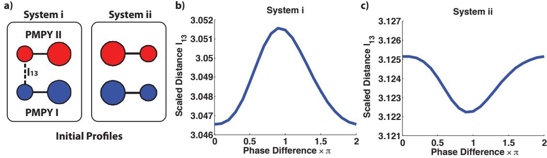
**Fig. 5.5** Two PMPYs swim from a parallel initial position. (a) With  $l_0 = 8$ ,  $l_{13}(0) = 10$ ,  $\psi_0 = 0$ , the initial profiles of system i and ii. (b) The relation between the scaled distance in the vertical direction between sphere 1 and 3 in system i after one cycle ( $l_{13}(1)$ ) and the phase difference  $\psi_0$ . (c) As in (b) but for system ii.
