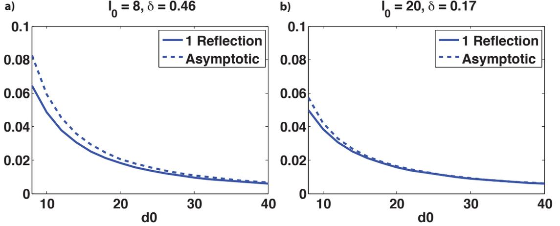
Fig. 5.4  $\hat{l}_{23}(1) - \hat{l}_{23}(0)$  for system i, with different values of  $l_0$  and  $d_0$ , where the translation is either calculated up to the first reflection (solid lines), or by asymptotic approximation to  $O(\delta)$  (dashed lines).
