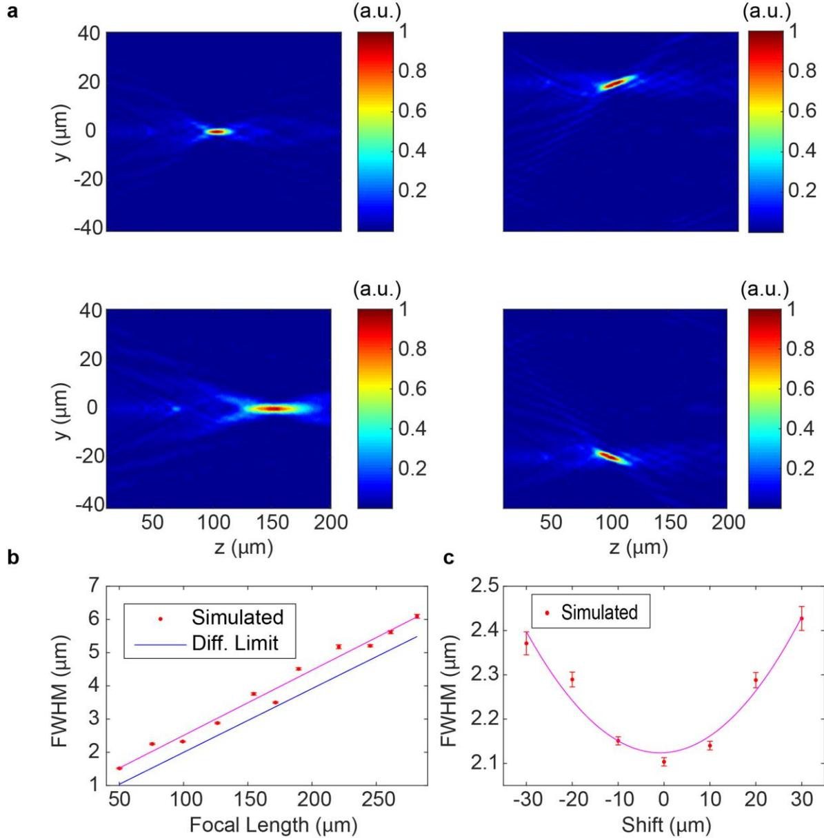
Figure 3: Tunable aspherical lenses: (a) FDTD-simulated intensity profiles for focal scanning on-axis (left) and in-plane (right) (b) Spot size as a function of focal length (c) Spot size as a
