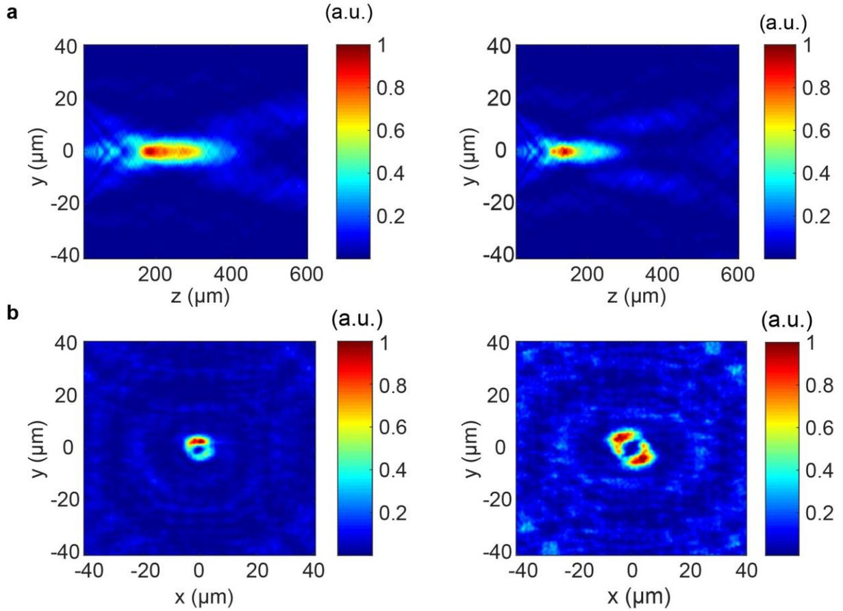
Figure 4: Tunable metasurface axicons and vortex beam generators: (a) Intensity profiles for axicons with  $\beta = 4^\circ$  (left) and  $\beta = 5^\circ$  (right) (b) Intensity profiles for a vortex beam generator with  $l = 1$  (left) and  $l = 2$  (right)
