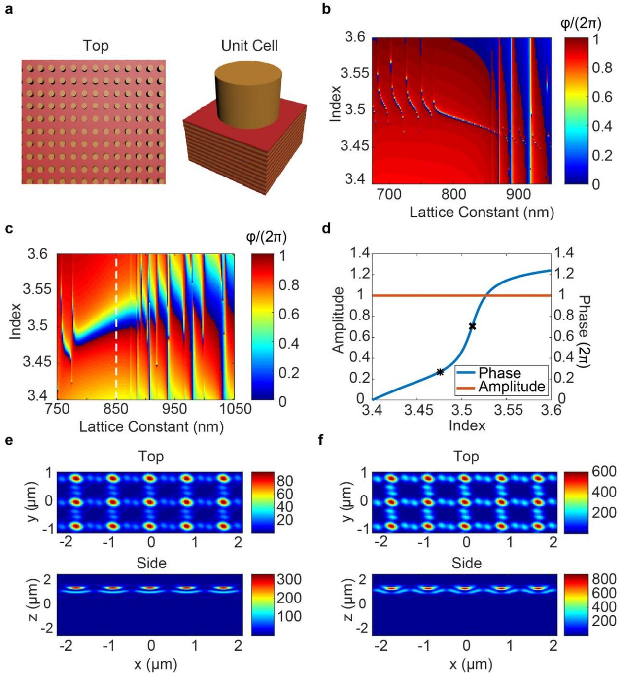
Figure 2: Design of scattering nanoparticles: (a) Top view schematic of a metasurface composed of nanoparticles atop a DBR with the unit cell shown, RCWA-calculated reflection coefficients as a function of index and lattice constant for rapid (b) and moderate (c) phase change regimes, (d) reflection coefficient for a fixed period corresponding to the white dashed line in (c) with phase
