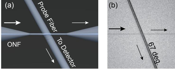
FIG. 2. (a) Schematic of probe fiber with respect to ONF. (b) Camera image of probe fiber and nanofiber on the ONF waist.
