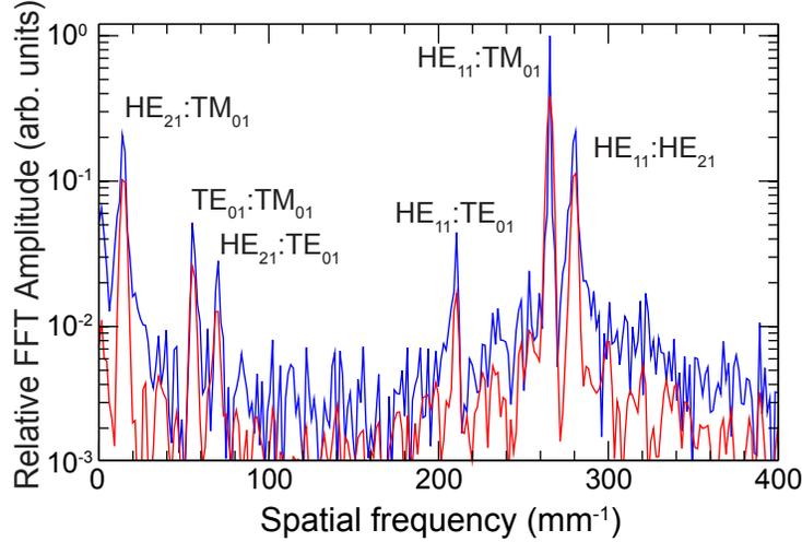
FIG. 6. FFT of a  $600 \mu\text{m}$  long segment of the data (waist of the ONF in Fig. 4). Note the logarithmic vertical scale. The blue trace is the raw data and the red has been multiplied by a Gaussian filter (see text for details).
