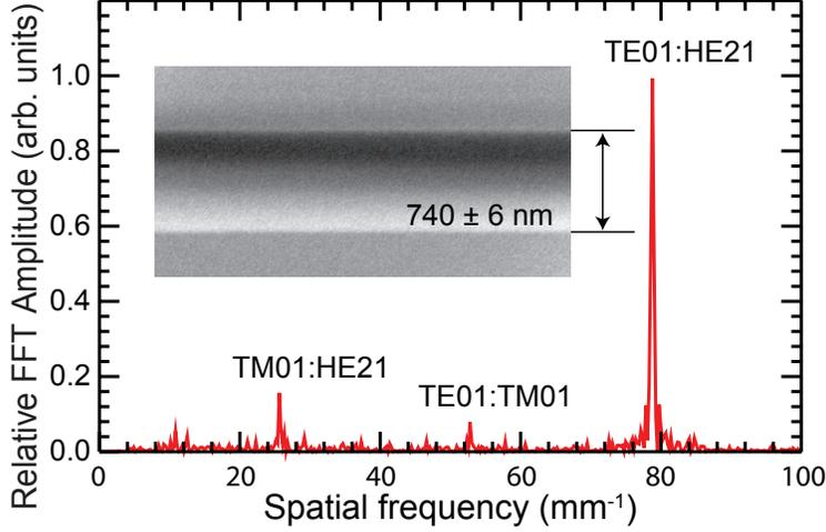
FIG. 7. Beat frequencies for the fiber shown in the inset SEM image. The low spatial frequency beat frequencies correspond to a fiber diameter of  $742 \pm 0.3$  nm, in agreement with the SEM measurement of  $740 \pm 6$  nm.
