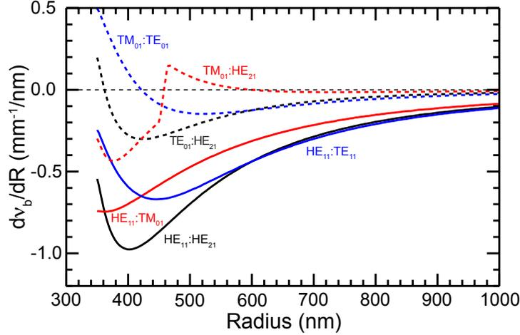
FIG. 5. Rate of change of the beat frequency with fiber radius. Note that the  $HE_{11} : HE_{21}$ ,  $HE_{11} : TE_{11}$ , and  $HE_{11} : TM_{01}$  have high sensitivity to radius near 400 nm.
