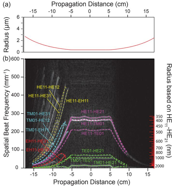
FIG. 4. (a) Design profile for ONF as a function of propagation distance. (b) Spectrograms of the data, along with calculated beat-frequency curves for a number of mode pairs as a function of propagation distance. Curves of the same color belong to the same family. The right axis on (b) shows the extracted radius corresponding to the  $HE_{11} : TM_{01}$  curve.
