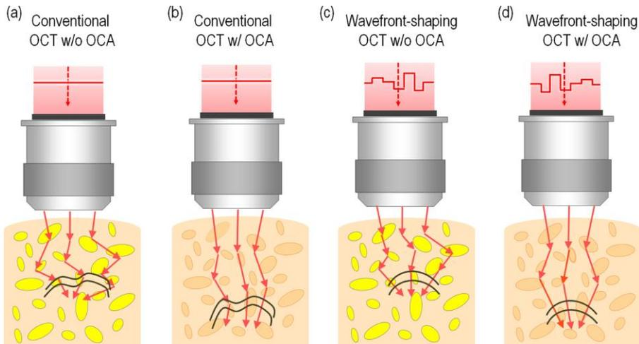
**Fig. 1** Principle of optical clearing agents and wavefront shaping in an OCT system. (a) Conventional OCT imaging. (b) After the application of OCAs, the overall scattering of the tissue is reduced. (c) Wavefront shaping in OCT. The optimal incident wavefront generates a tight focus inside the tissue. (d) Combined effect of OCAs and wavefront shaping. Maximal penetration depth can be achieved with reduced scattering of the sample and optimal incident light field.
