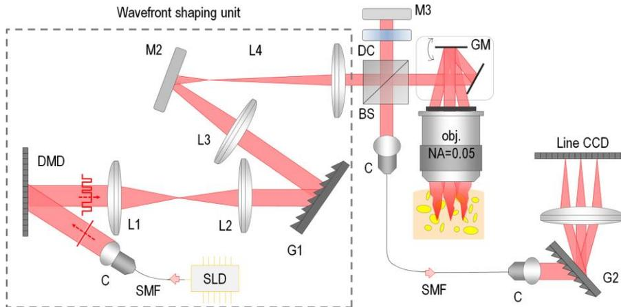
**Fig. 2** Experimental setup. Gray dashed rectangular area: wavefront shaping unit: SLD - super-luminescent diode, DMD - digital micro-mirror device, G1 - dispersion compensating grating; BS - beam splitter, DC - dispersion compensator, GM - galvo mirror, G2 – spectral OCT grating; C – collimators, L - lenses, M - mirrors, SMF – single mode fiber. The intensity modulation after the DMD is not to scale.
