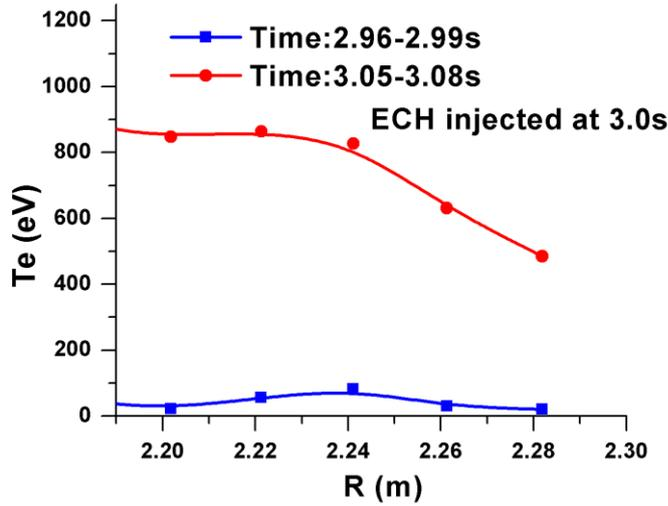
**Fig.13** Profiles of electron temperature at edge region in shot 16478. ECH is injected at 3.0s. The last closed flux surface is at about  $R=2.24\text{m}$  estimated by EFIT.
