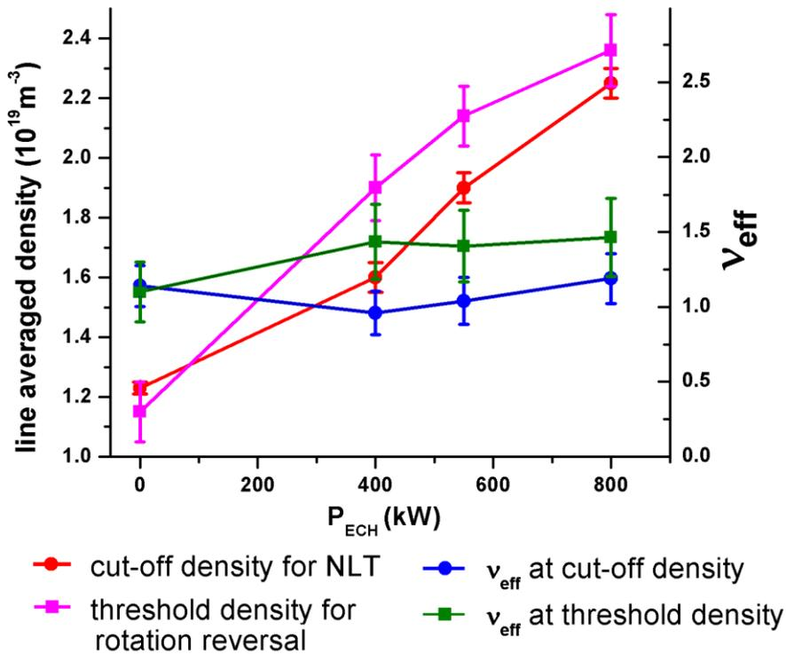
**Fig.4** The cut-off density for NLT and threshold density for rotation reversal in ECH power scan shots. The normalized effective collisionality ( $v_{eff}$ ) at  $\rho \sim 0.5$  at cut-off density and threshold density is also plotted in this figure.
