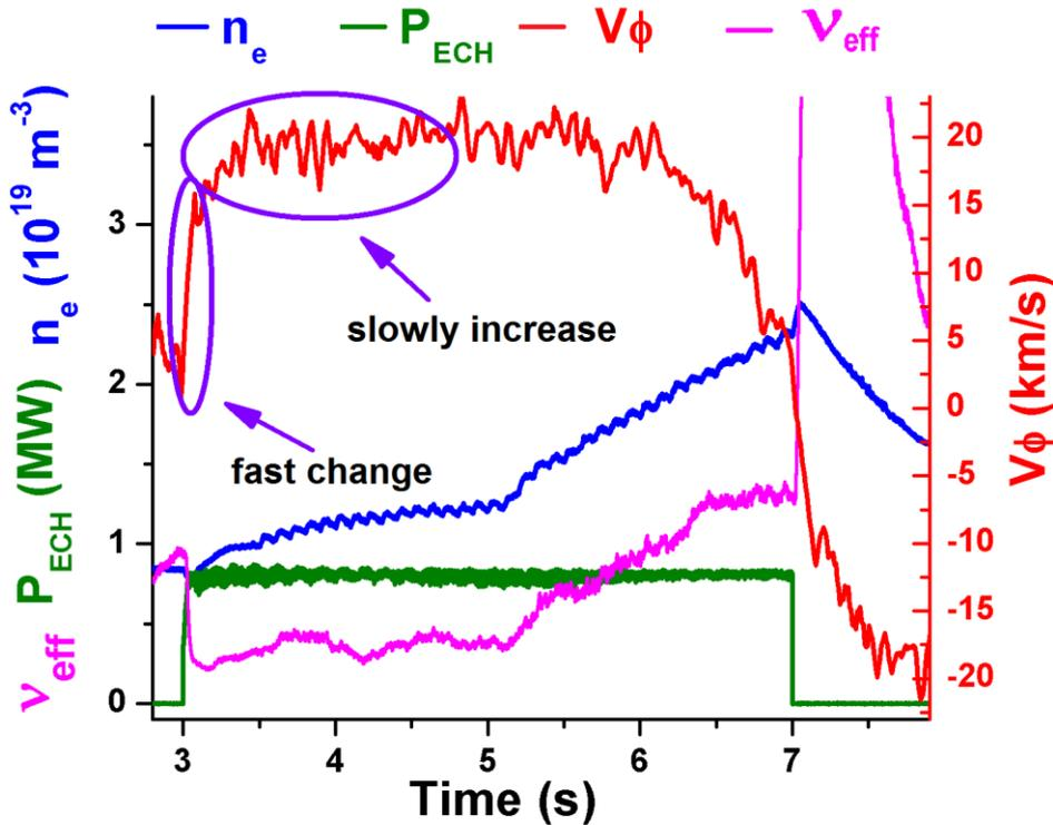
Fig.12 Temporal evolution of core  $V_\phi$ , line averaged density, power of ECH, and  $v_{\text{eff}}$  at  $\rho \sim 0.5$  in shot 16478
