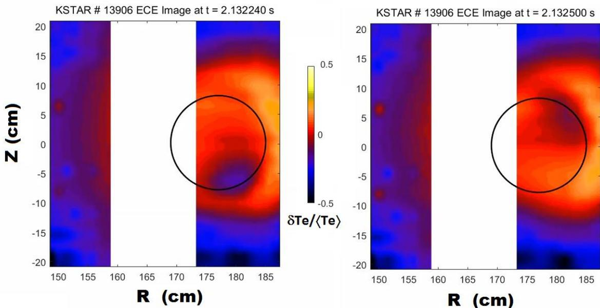
**Fig.6** 2D electron temperature fluctuation image from ECEI during NLT in ECH plasma. The time interval for the two image is 0.26ms. The pattern of temperature increasing area (red color) is very clear. The black circle represent the approximate location of  $q=1$  surface. The blue spot at the  $q=1$  surface is the  $m/n=1$  island, which is in different location at different time due to the general rotated property of MHD island.
