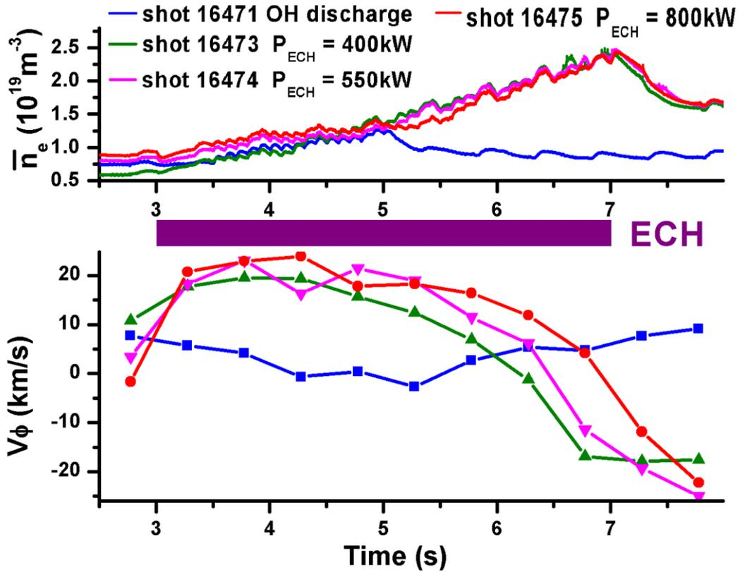
**Fig.5** Temporal evolutions of core  $V_\phi$  (measured by CES) and line averaged density for OH plasma and ECH plasmas with power scan
