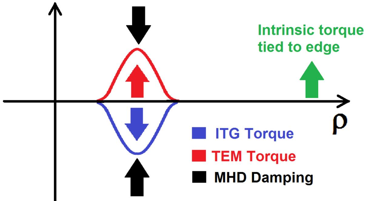
Fig.9 Cartoons shows the torque and damping source for intrinsic rotation in KSTAR
