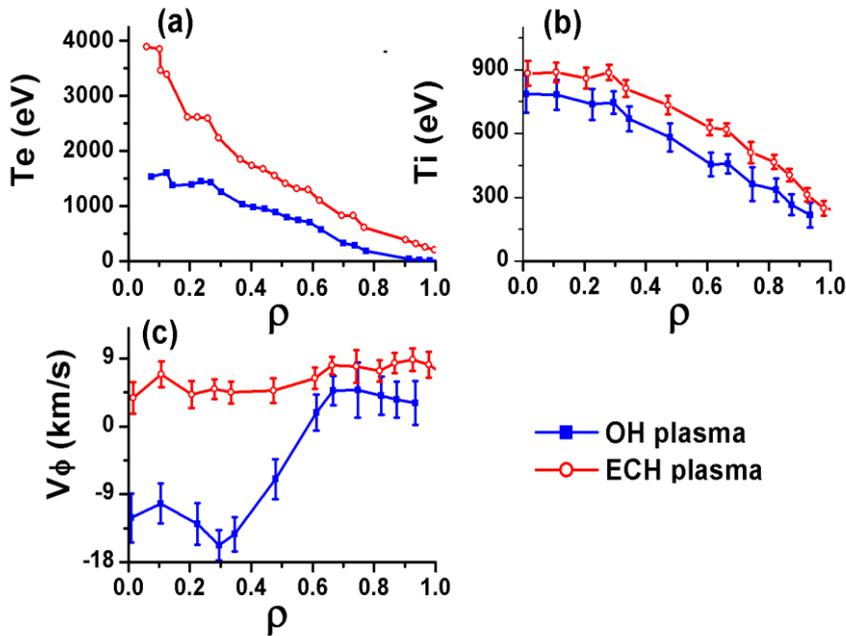
**Fig.2** Profiles of macro parameters for two ECH and OH discharges in fig.1 at same density. (a) electron temperature, (b) ion temperature, (c) toroidal rotation velocity,
