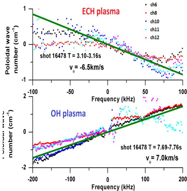
**Fig.8** The cross-phase spectra of MIR. Here, 5 dispersions for centre channels with respect to channel 9 are overlapped. The poloidal velocity is estimated from the inverse of the slope of a fitted line (green color) on the dispersion relation. The measurement position is about  $\rho \sim 0.15$  for ECH plasma and  $\rho \sim 0.35$  for OH plasma.
