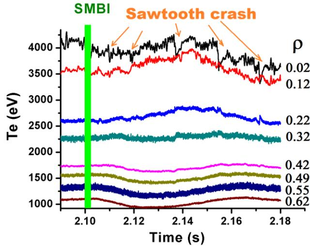
**Fig.3** Temporal evolutions of electron temperature measured at different radii in the ECH plasma for the first SMBI pulse in fig.1.
