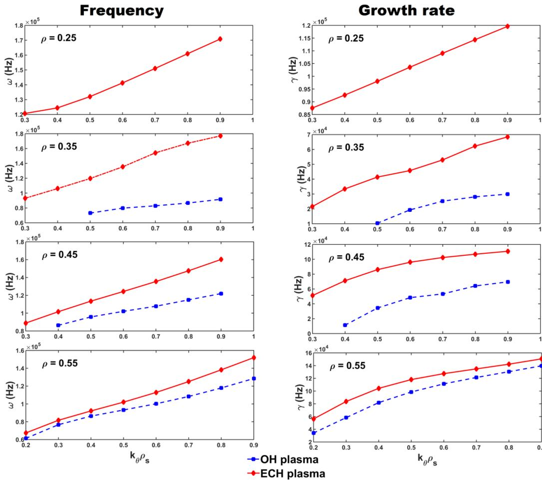
**Fig.14** The mode frequency and growth rate for OH plasma and ECH plasma. The experimental parameters for simulation are come from fig.3. Positive mode frequency means the modes in the electron diamagnetic direction; negative mode frequency means the modes in the ion diamagnetic direction.
