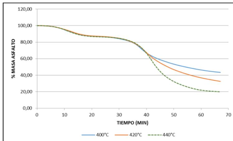
**Figure 13.** Curve thermogravimetric asphalt without catalyst reaction temperatures
