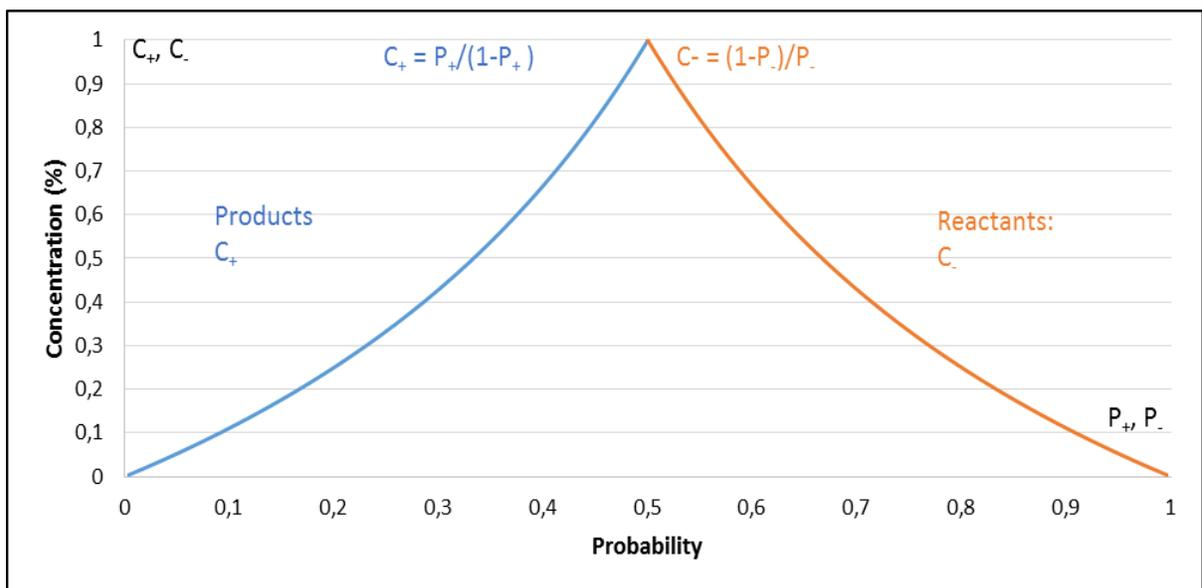
**Figure 1.** Showing the concentrations of reactants and products in function on the value of probability (blue:  $C_+$  Vs  $P_+$ , orange:  $C_-$  Vs  $P_-$ ) for an irreversible first order reaction where reactants  $\rightarrow$  products.
