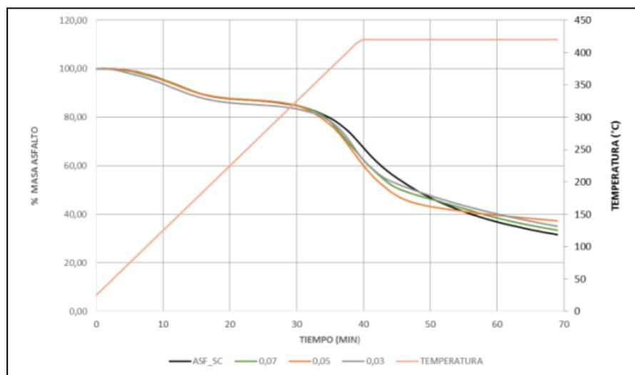
**Figure 15.** Thermogravimetric curve at 420 ° C
