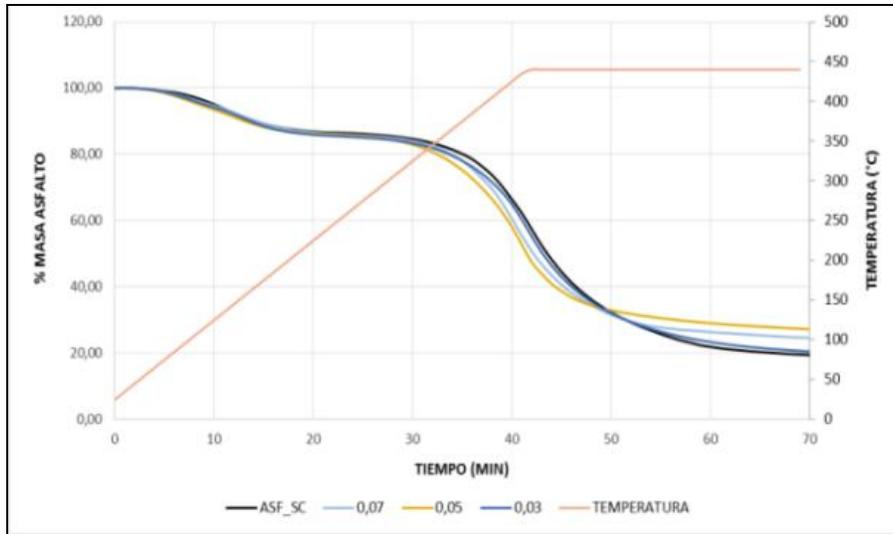
**Figure 16.** Thermogravimetric curve at 440 ° C
