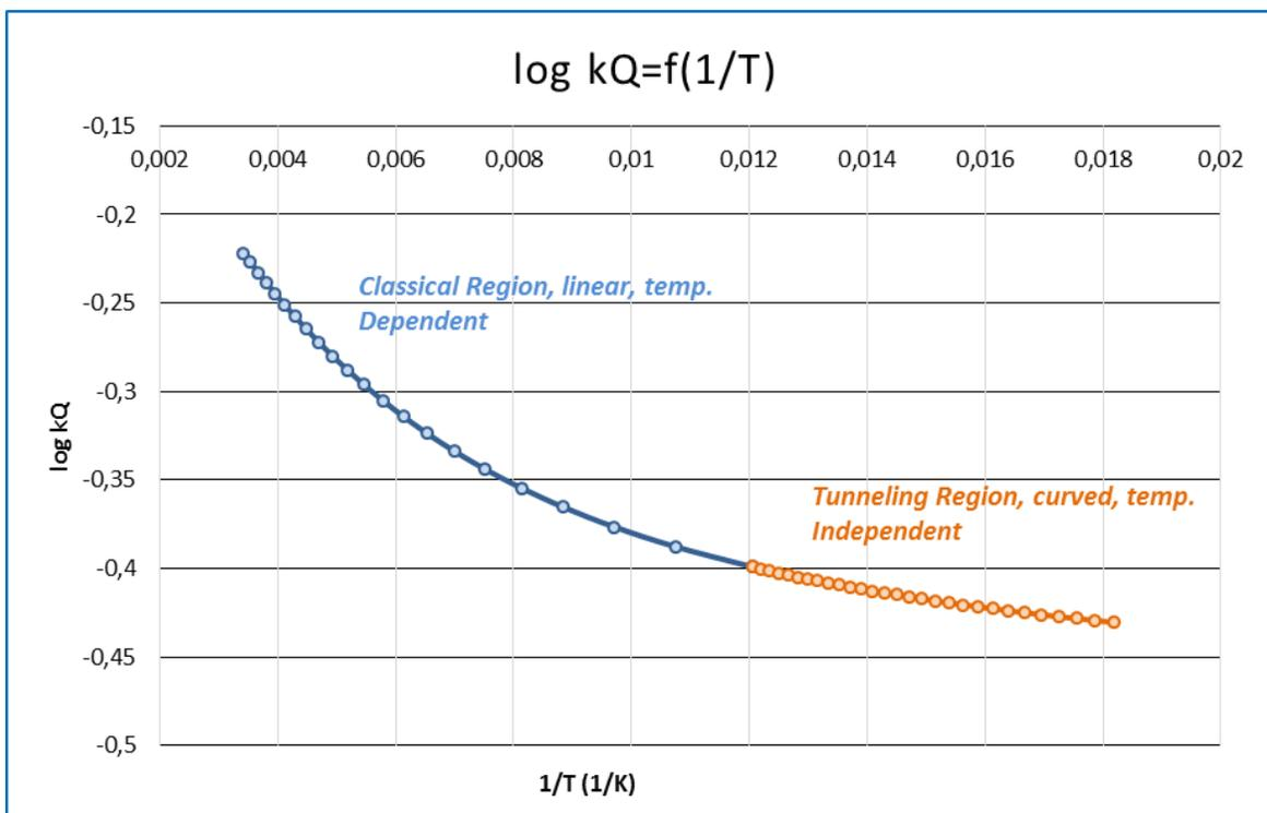
**Figure 3.** Arrhenius Quantum Equation. Theoretical and experimental foundations of hydrogen production. The temperature independence in the range (54, 83) K is showed (orange line); where the studied curve takes an evident linear trend. Furthermore, this theoretical set contains our experimental set of  $82 \pm 1$  K, giving us the coherence between theory and experiment.
