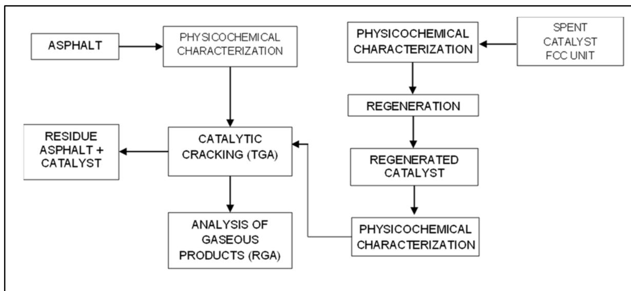
**Figure 5.** Flow diagram of the experimental setup to the catalytic process
