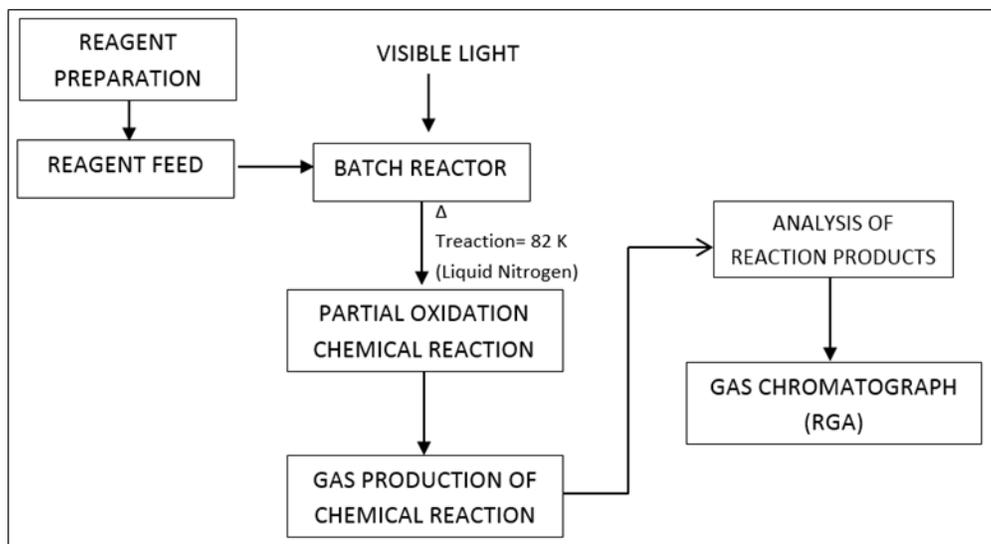
**Figure 4.** Flow diagram of the experimental setup.
