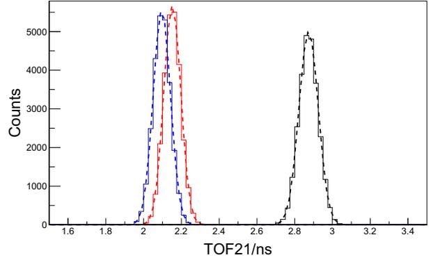
Fig. 6. TOF21 distributions in cases without correction (black line), with only the walk-effect correction (blue line) and with both walk-effect and position correction (red line). The Gaussian fits (dashed lines) for the three cases show a standard deviation ( $\sigma$ ) of 51 ps, 46 ps and 45 ps, respectively.
