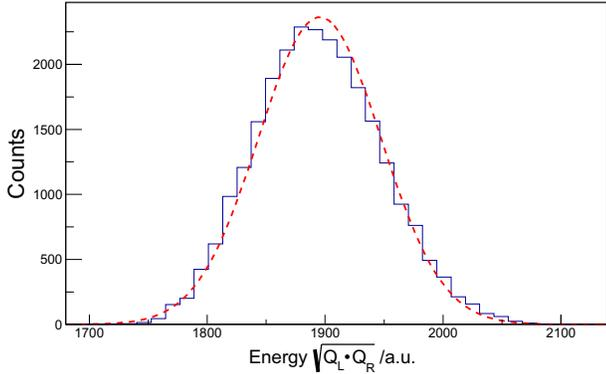
Fig. 8. Energy resolution of PL1 is about 3% ( $\sigma$ ) deduced by Gaussian fit.
