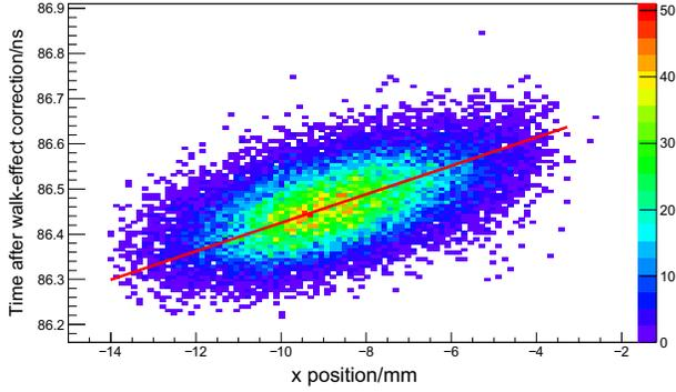
Fig. 4. Position dependence of the timing. The red line indicates the linear fitting.
