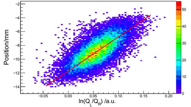
Fig. 9. Correlation between position and  $\ln(Q_L/Q_R)$ . The linear correlation is indicated by the red line.
