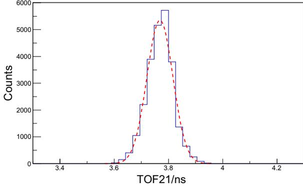
Fig. 7. TOF21 distribution (solid line) using the data registered by MULTITDC. A Gaussian fit is indicated by the dashed line.
