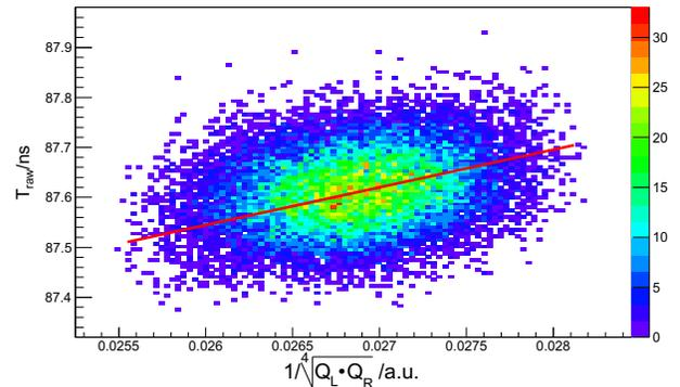
Fig. 2. Pulse-height dependence of the timing. The red line indicates the linear fitting.
