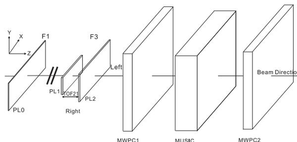
Fig. 1. Schematic view of the experimental setup for the TOF test experiment at RIBLL2.
