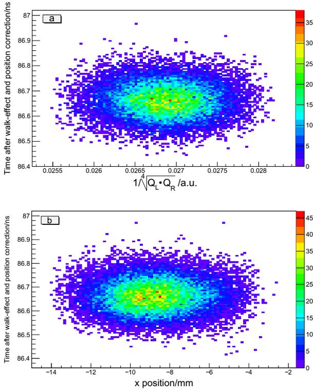
Fig. 5. Timing after walk-effect and position correction as a function of pulse-height (a) and hitting position (b).
