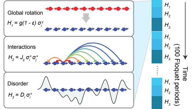
FIG. 1: **Floquet evolution of a spin chain.** Three Hamiltonians are applied sequentially in time: a global spin flip of nearly  $\pi$  ( $H_1$ ), long-range Ising interactions ( $H_2$ ), and strong disorder ( $H_3$ ). The system evolves for 100 Floquet periods of this sequence.
