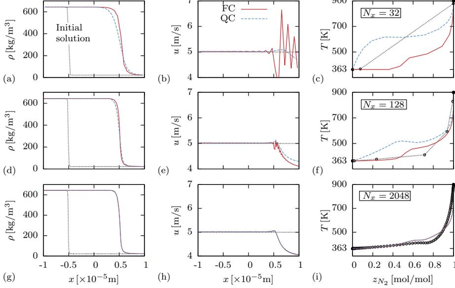
FIGURE 1. FC-F and QC-F results for 1-D advection-diffusion test case for different grid resolutions. Left column: density profiles in physical space; center column: velocity profiles in physical space; right column: temperature profiles in mixture space; dotted lines are the initial profiles.
