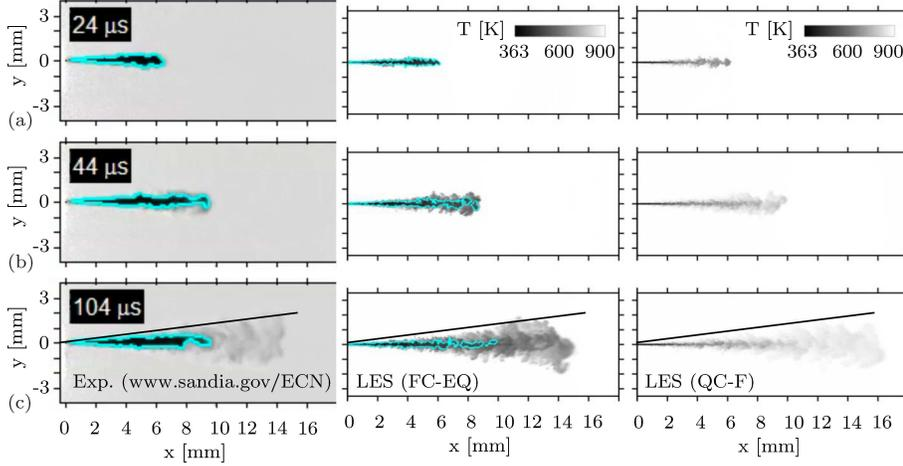
FIGURE 2. Temporal sequence of the injection event. Left column: experimental data of Pickett *et al.* (2011); center column: LES with FC-EQ; right column: LES with QC-F. Liquid penetration length is illustrated by a  $LVF = 0.15\%$  iso-contour.
