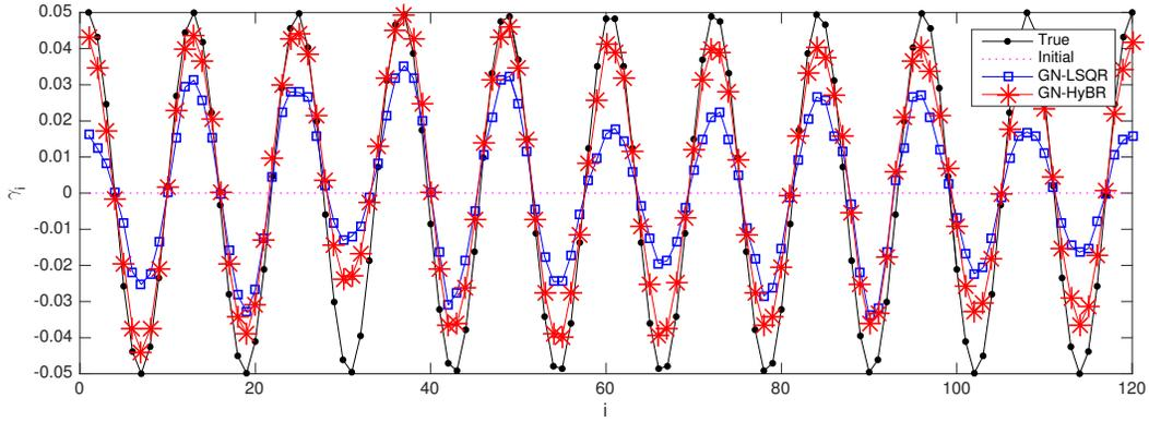
Figure 6: Motion parameters. The black, solid line corresponds to true motion parameters  $\gamma^{\text{true}}$  for each transducer given by  $\gamma_i = 0.05 \cos(10 \phi_i)$ . The initial guess assumes no motion, thus  $\gamma^{(0)} = \mathbf{0}$  (dotted line). Computed motion parameters after 6 Gauss-Newton iterations where LSQR and HyBR were used to solve the linear subproblem are provided in blue squares and red stars respectively.
