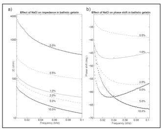
Figure 1. Effect of NaCl loading on ballistic gelatin impedance magnitude (a), and phase (b).
