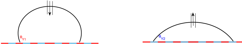
FIG. 6.1. The advancing and receding contact angles on a chemically patterned surface.
