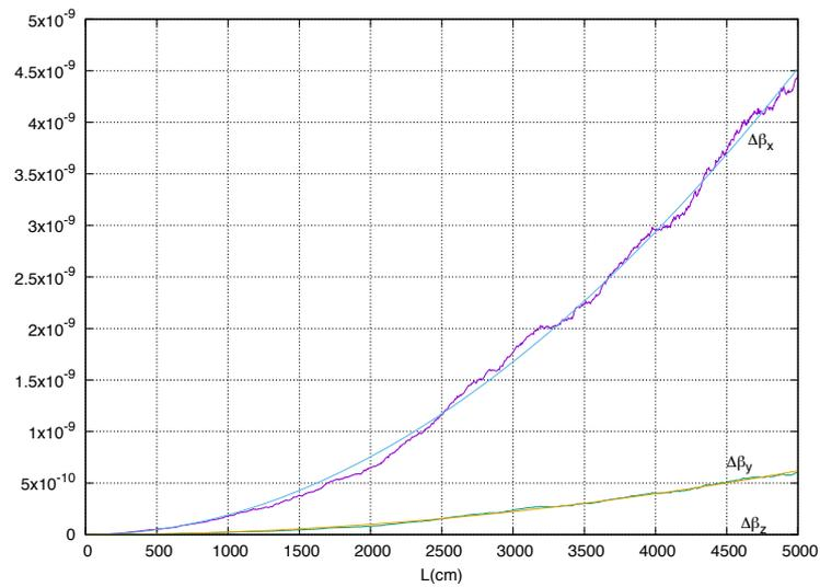
Figure 1: Difference of the normalized velocity components as a function of the undulator length.
