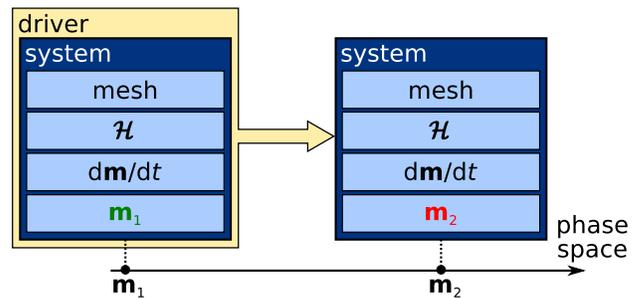
FIG. 1. A schematic representation of our micromagnetic model. The system object is completely defined with: (i) mesh, (ii) Hamiltonian  $\mathcal{H}$ , (iii) dynamics equation  $d\mathbf{m}/dt$ , and (iv) magnetisation configuration  $\mathbf{m}$ . The driver is “driving” (moving) the system through phase space by changing its magnetisation from  $\mathbf{m}_1$  to  $\mathbf{m}_2$ .
