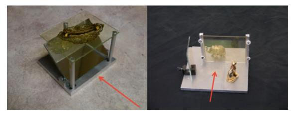
**Figure 2** Plate/object supports PO1 (left) and PO2 (right). The arrows indicate the orientation of the diverging laser beams. The plate/object supports are placed far enough from the lasers so that the maximum surface of the 4"x5" plates are exposed. PO2 is used for single shot reflection/transmission holograms: a reflection hologram of the elephant and a transmission hologram of the cat are produced simultaneously.
