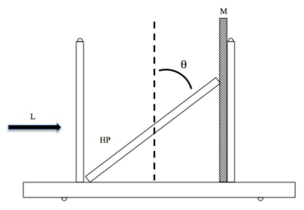
**Figure 4** Experimental setup for the realization of a holographic diffraction grating with the plate/object support PO1. The laser beam L is coming from the left side. The holographic plate HP is leaned against the mirror M, emulsion on the mirror side. The inclination of HP can be varied by changing the position of the rear post.
