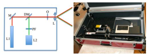
**Figure 1** Diagram of the optical setup inside the case (left) and its photography (right). L1: 20 mW 632.8 nm HeNe laser; L2: 20 mW 532 mn DPSS laser; PF: polarizing filter; DM: dichroïc mirror; M : front surface mirror; O : obturator; L : lens. On the photography, the exit port and the lens L are located on the upper left side of the case. A small case contains the supplementary material and is placed on the top of the lasers power supplies.
