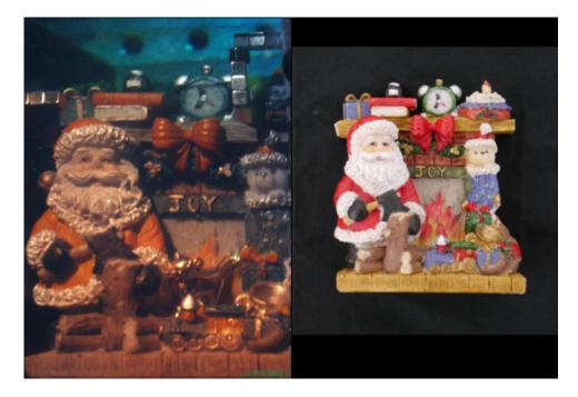
Figure 3 Two-colours (red/green) hologram of a Christmas toy (left), and the original object (right).
