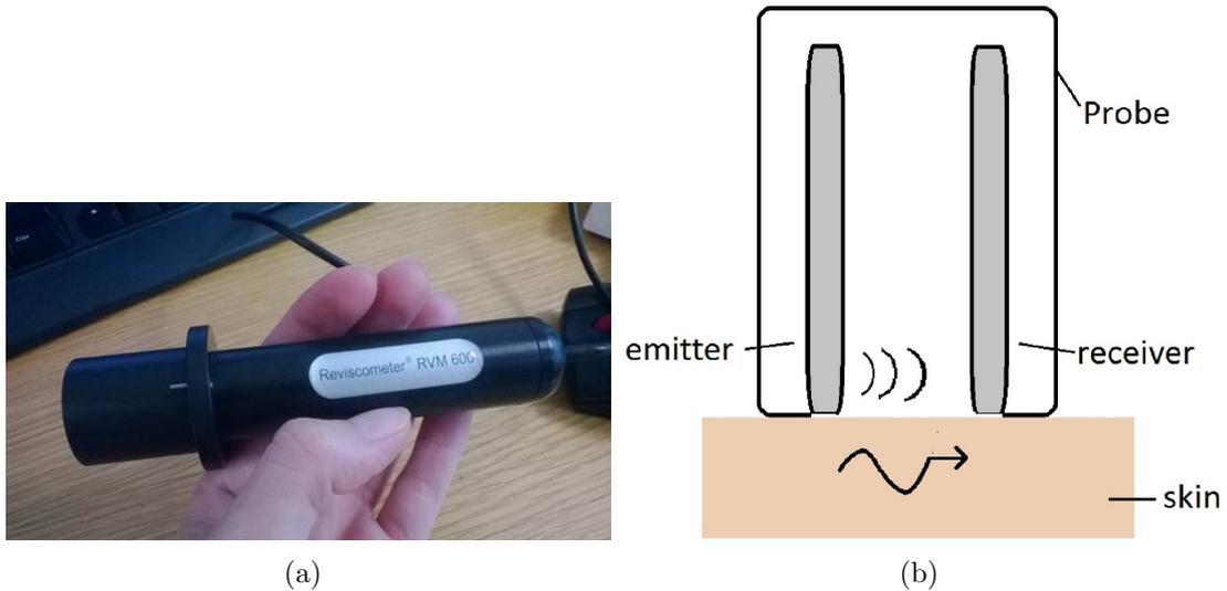
Figure 1: (a) Reviscometer device<sup>®</sup>. (b) Mechanism of operation.
