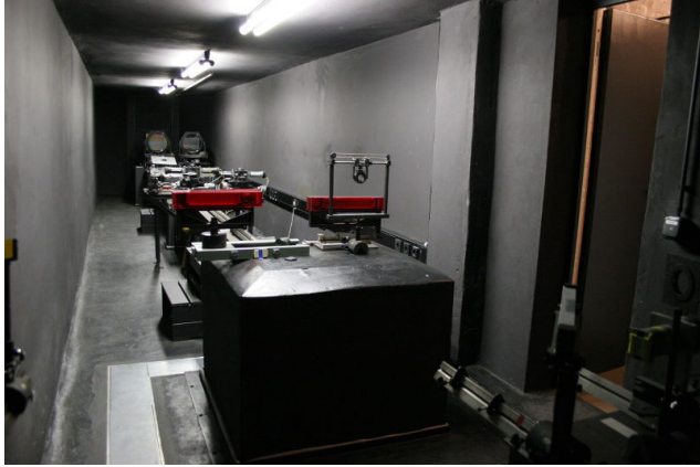
Fig. 7 Interior of the spectrograph chamber with the twin high-resolution spectrographs. Large-format gratings are located in the back behind collimating lenses used in double path. An optical bench on a separate foundation supports the spectrograph optics and facilitates insertion of additional optical elements. Turning mirrors (one in the foreground and two with red protective plastic covers) redirect the light to (polarization) optics or CCD cameras.
