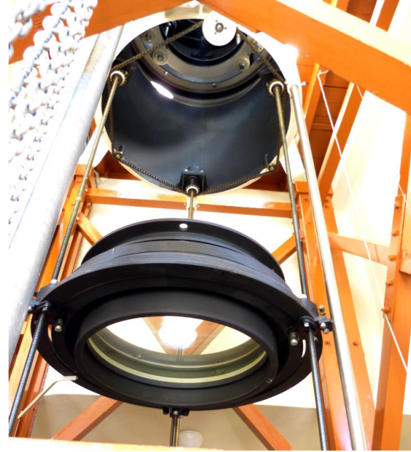
Fig. 6 Mounting of the 60-centimeter doublet lens with gearing mechanism to adjust the focus position.
