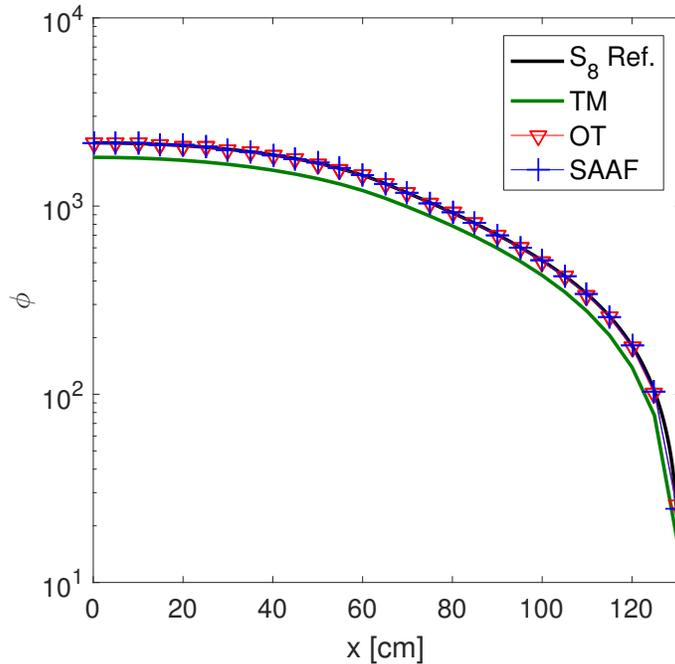
Figure 3: Natural carbon test with neutron at RT with mesh size  $h = 5$  cm.
