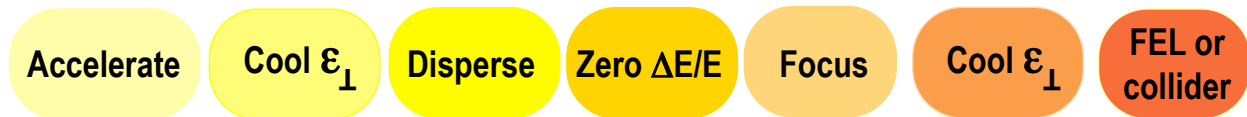
FIGURE 1. Stages of Laser-Plasma Staged FEL: acceleration, cooling transverse degrees of freedom, dispersing the beam, monochromatization, focusing, one more transverse cooling stage, and sending the cooled beam to an FEL undulator or, for use in a collider.
