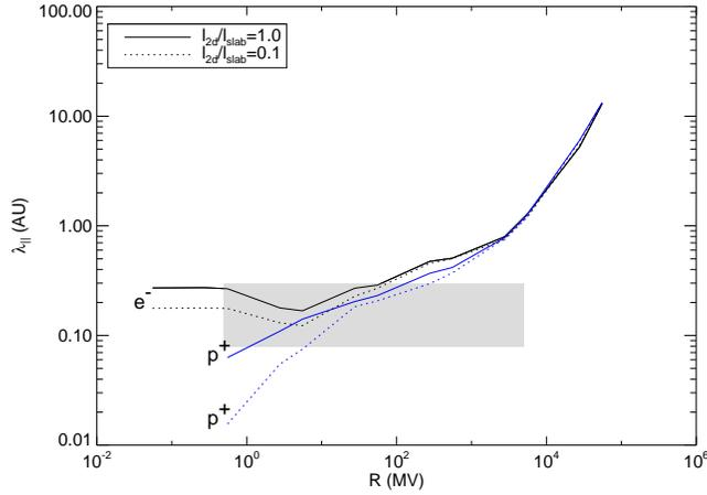
Fig. 14.— The parallel mean free path versus magnetic rigidity for two-component turbulence, the NADT model, and  $\delta B/B_0 = 0.5$ . We have shown results for different values of the two-dimensional bendover scale  $l_{2D}$ . The shaded band represents the Palmer (1982) consensus range.
