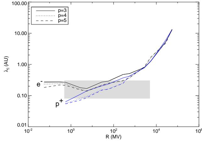
Fig. 11.— The parallel mean free path versus magnetic rigidity for two-component turbulence, the NADT model, and  $\delta B/B_0 = 0.5$ . We have shown results for different values of the dissipation range spectral index  $p$ . The shaded band represents the Palmer (1982) consensus range.
