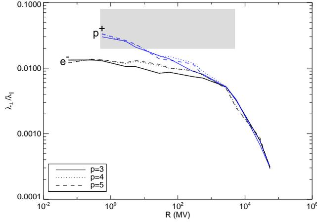
Fig. 13.— The ratio of perpendicular and parallel mean free paths versus magnetic rigidity for two-component turbulence, the NADT model, and  $\delta B/B_0 = 0.5$ . We have shown results for different values of the dissipation range spectral index  $p$ . The shaded band represents the Palmer (1982) consensus range.
