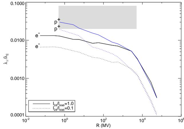
Fig. 16.— The ratio of perpendicular and parallel mean free paths versus magnetic rigidity for two-component turbulence, the NADT model, and  $\delta B/B_0 = 0.5$ . We have shown results for different values of the two-dimensional bendover scale  $l_{2D}$ . The shaded band represents the Palmer (1982) consensus range.
