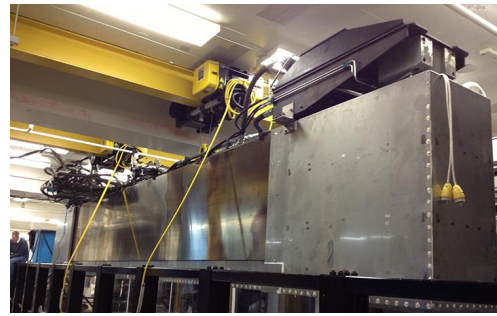
Figure 3: Perspective view of the Ship Boundary Layer Simulator (SBL) and the water tank and a photo of the belt device being lowered into the tank.
