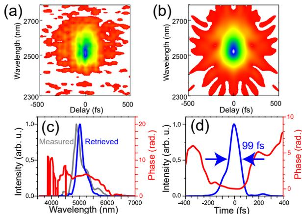
FIG. 3. SHG-FROG characterization of the 99-fs,  $5.2\text{-}\mu\text{m}$  pulses generated in a 4-mm-thick ZGP crystal. Measured (a) and reconstructed (b) SHG-FROG traces. (c) Retrieved spectrum (blue line), retrieved spectral phase (red line), and measured spectrum (gray line). (d) Retrieved temporal pulse profile (blue line) and temporal phase (red line).
