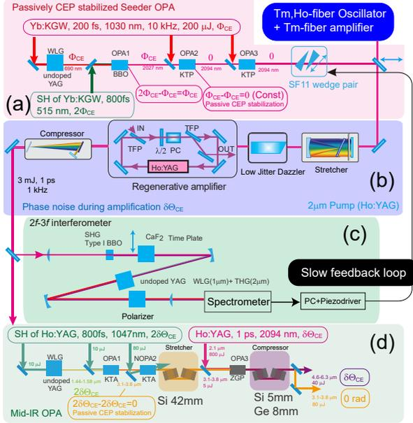
FIG. 1. Optical layout consisting of (a) a passively CEP stabilized seeder OPA, (b) a CEP stabilized  $2 \mu\text{m}$  pump (Ho:YAG), (c) a  $2f$ - $3f$  interferometer, and (d) a CEP stabilized MIR OPA.
