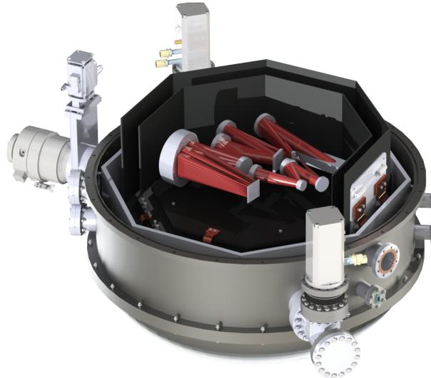
Figure 9. CAD rendering of the iLocater cryostat showing spectrograph optics located inside of a nested set of radiation shields and stainless steel vacuum jacket.
