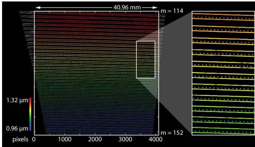
Figure 6. iLocator's spectral format showing all 39 orders and three fiber spectral traces. An ultra-compact design generates diffraction-limited performance across the  $\lambda=0.97\text{-}1.30\ \mu\text{m}$  range. An H4RG ( $4096 \times 4096$  pixels) captures the Y-band and 85% of J-band.
