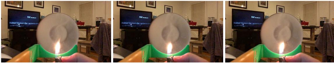
FIG. 5. Image sequence of burning butane lighter. The magic of OpenSchlieren does not translate well when displaying still images from the video sequence. Video sequence is available on YouTube at <https://youtu.be/NQ5LPR5koTA>.
