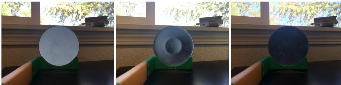
FIG. 4. Image of misaligned business card, from left to right: first, white part of card in imaged focus; second, properly aligned system; third, black part of business card in focus.
