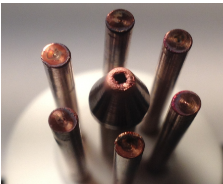
Figure 15. Results of erosion processes in MPC after 10^3 launches.
